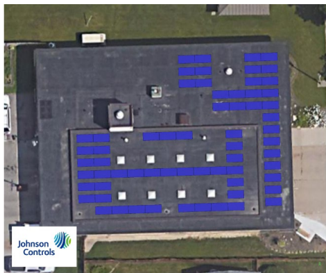
Fire Station #1: 36 kW
