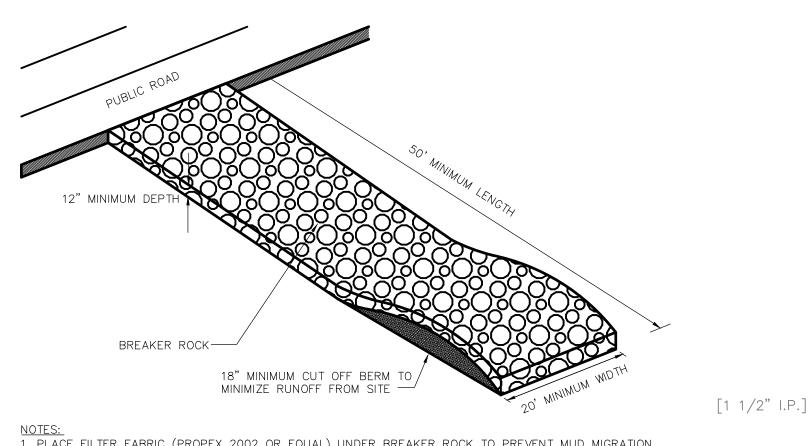
1. PLACE FILTER FABRIC (PROPEX 2002 OR EQUAL) UNDER BREAKER ROCK TO PREVENT MUD MIGRATION 2. ENTRANCE MUST BE MAINTAINED REGULARLY TO PREVENT SEDIMENTATION ON PUBLIC ROADWAYS. FUGITIVE ROCK WILL BE REMOVED FROM ADJACENT ROADWAYS DAILY OR MORE FREQUENTLY AS NECESSARY.
