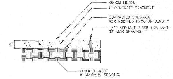
4" CONCRETE PAVING AND JOINTING
