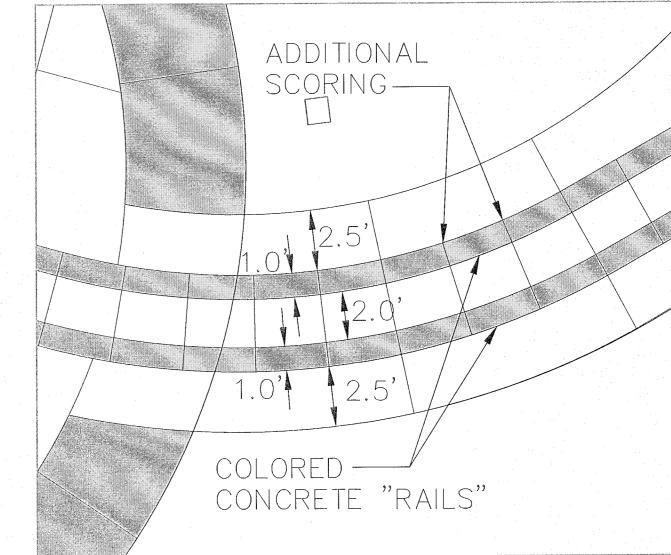
RAILROAD TRACK PAVING PLAN SCALE: 1/4"=1'-0"
