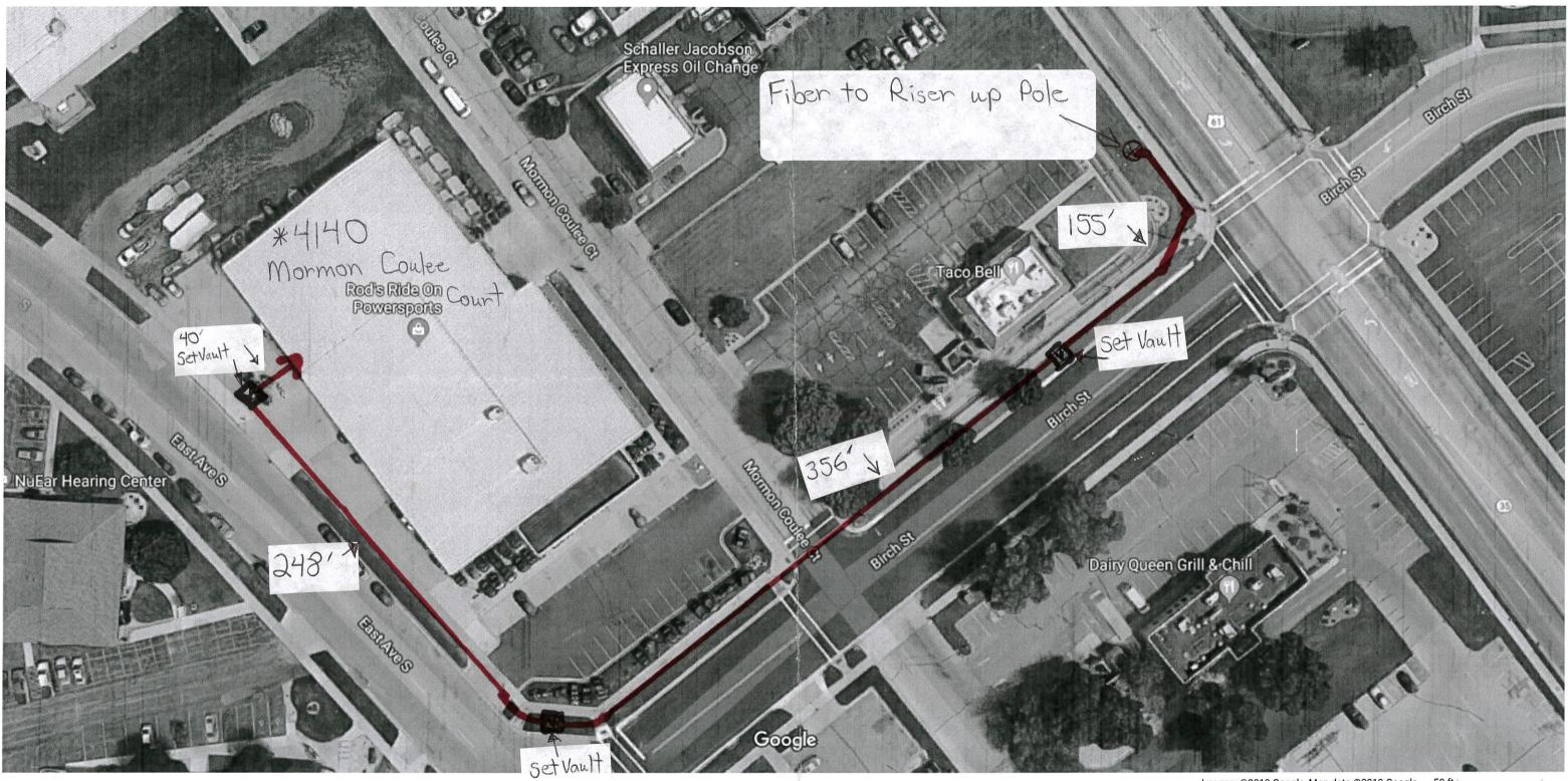
800 feet - Directional Bore @ 40" Deep placing 2" Duct a Fiber Optic Line to 4140 Mormon Coulee Ct. setting 3 Ground Flush Vaults
