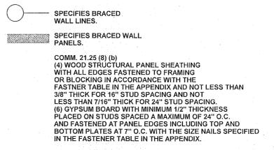
NOTE: REFER TO THE WISCONSIN (UDC) COMM. 21.25 FOR THE COMPLETE UNDERSTANDING OF THE BRACED WALL CODE.
