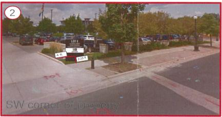
Sign to be placed 4ft from inside edge of driveway, and 2.25ft from inside edge of sidewalk towards brick wall. Grass area is 52" wide from brick wall to inside edge of sidewalk
