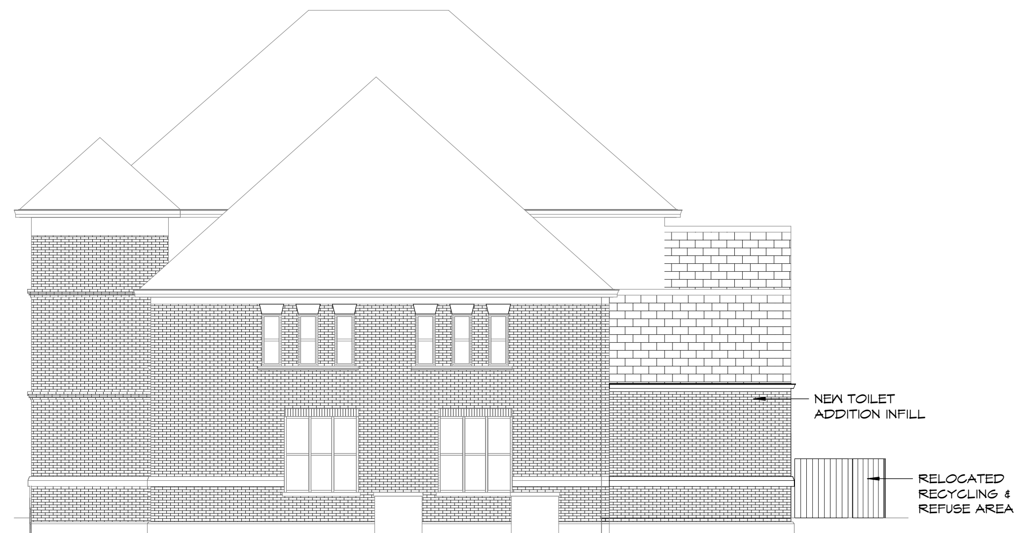
6 EAST ELEVATION - TOILET ADDITION 1/8" = 1'-0"
