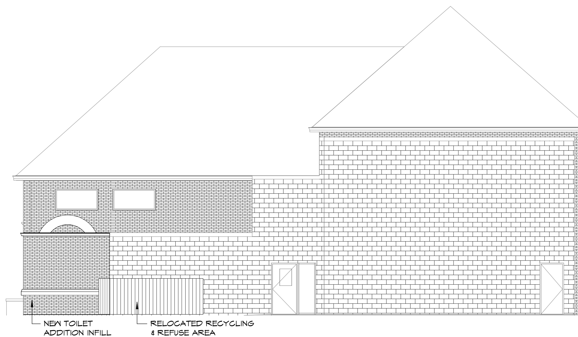
7 NORTH ELEVATION - TOILET ADDITION 1/8" = 1'-0"
