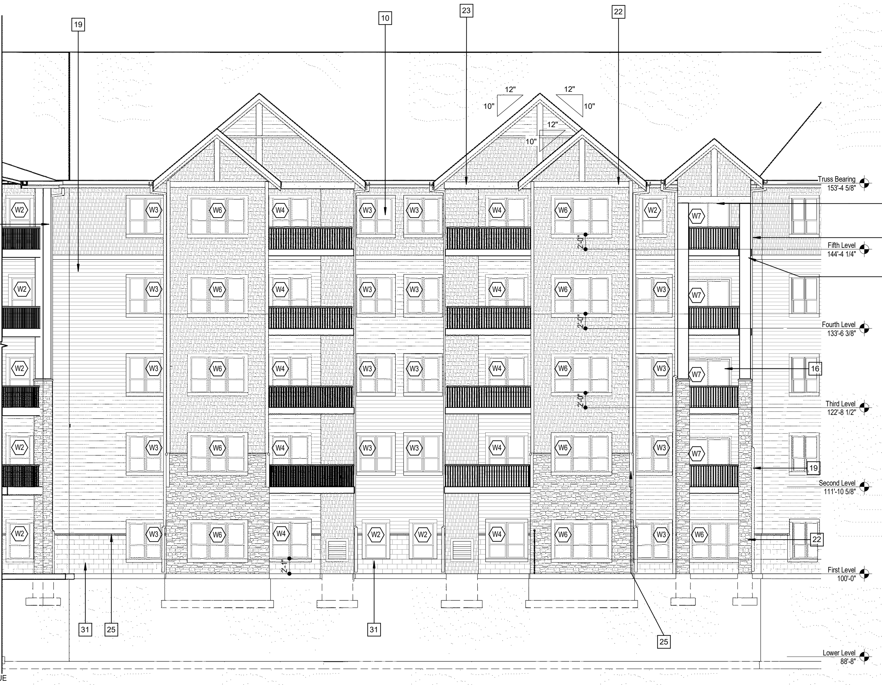
2 A3.3 EXTERIOR ELEVATION- AREA C (SE) 1/8" = 1'-0"
