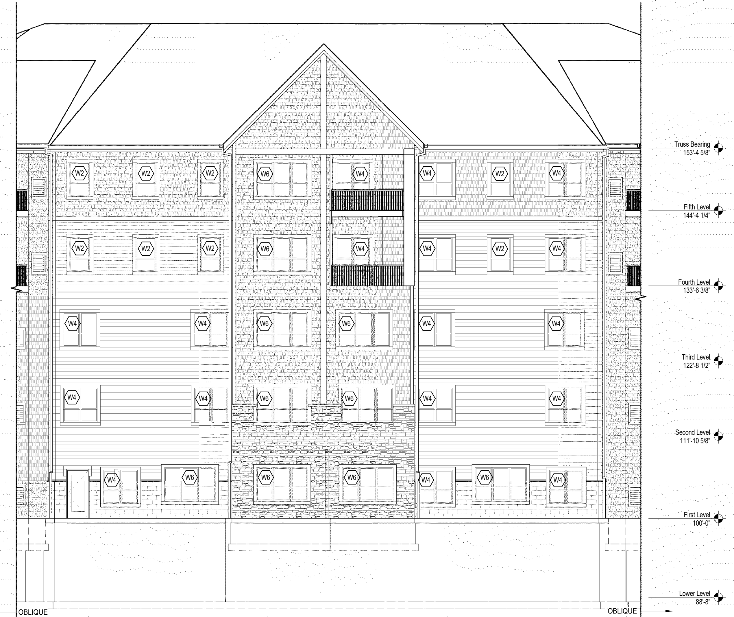
2 A3.5 EXTERIOR ELEVATION- AREA C (W) 1/8" = 1'-0"
