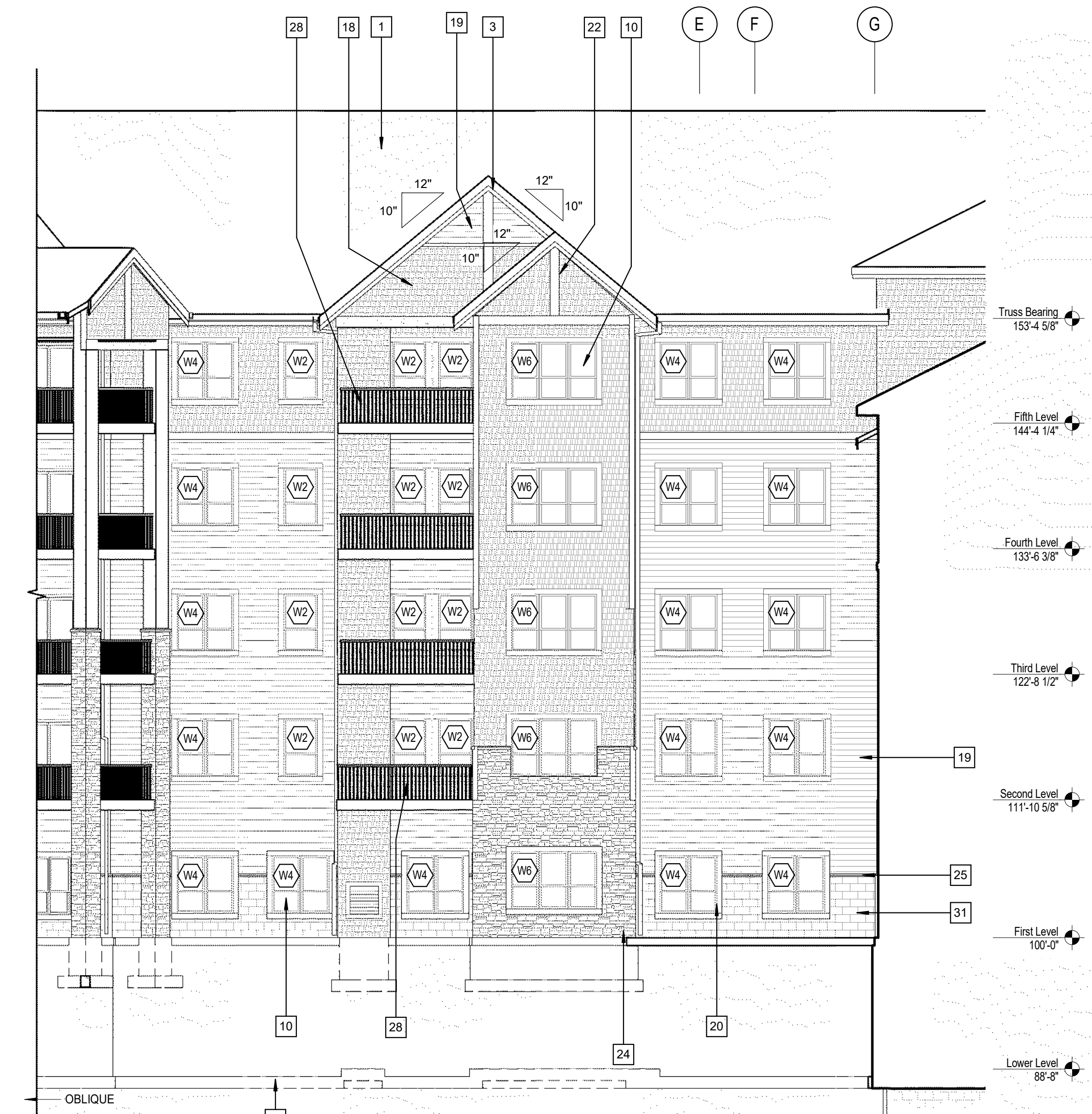
1 A3.3 EXTERIOR ELEVATION- AREA C (S) 1/8" = 1'-0"
