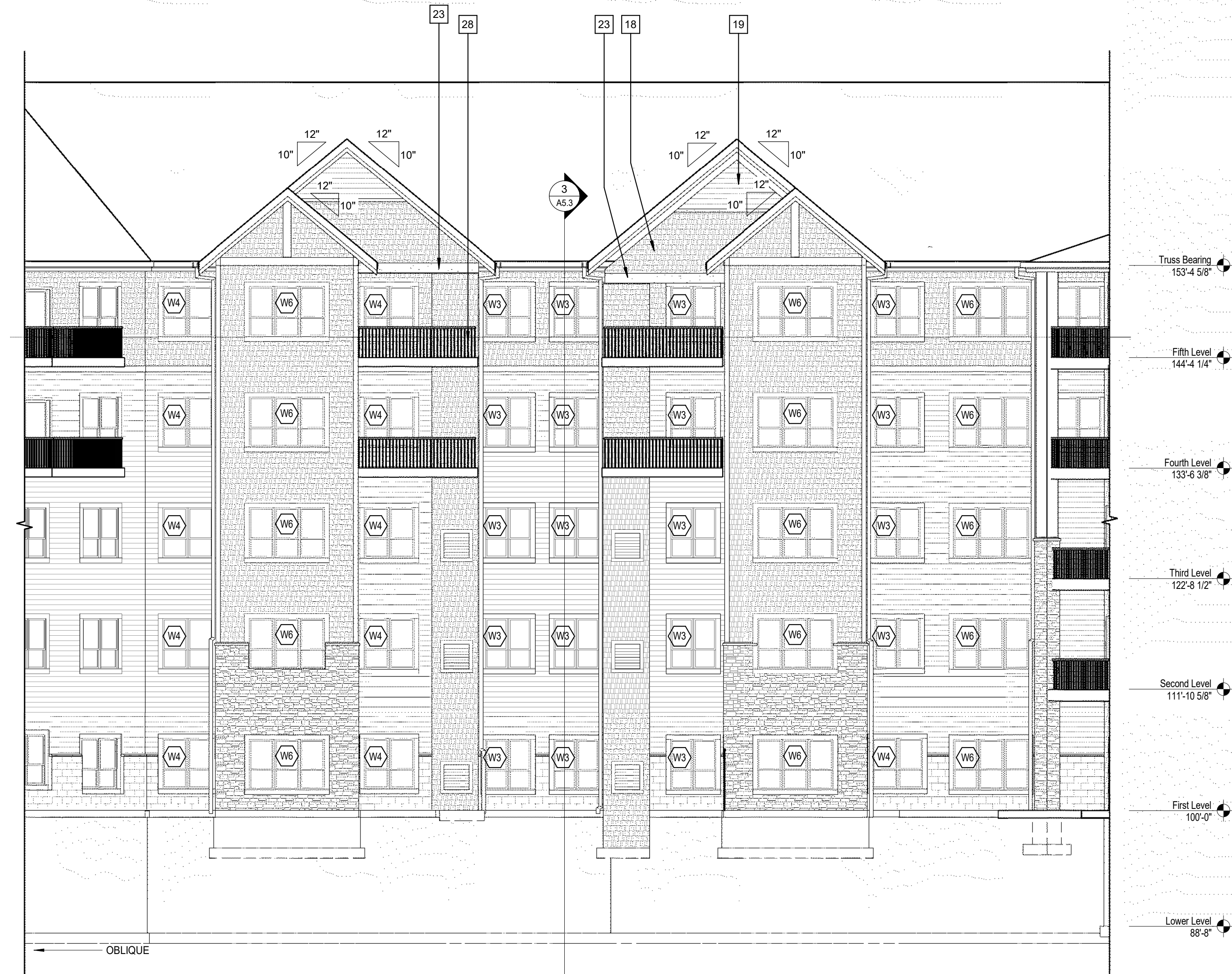
4 A3.3 EXTERIOR ELEVATION- AREA D (NE) 1/8" = 1'-0"
