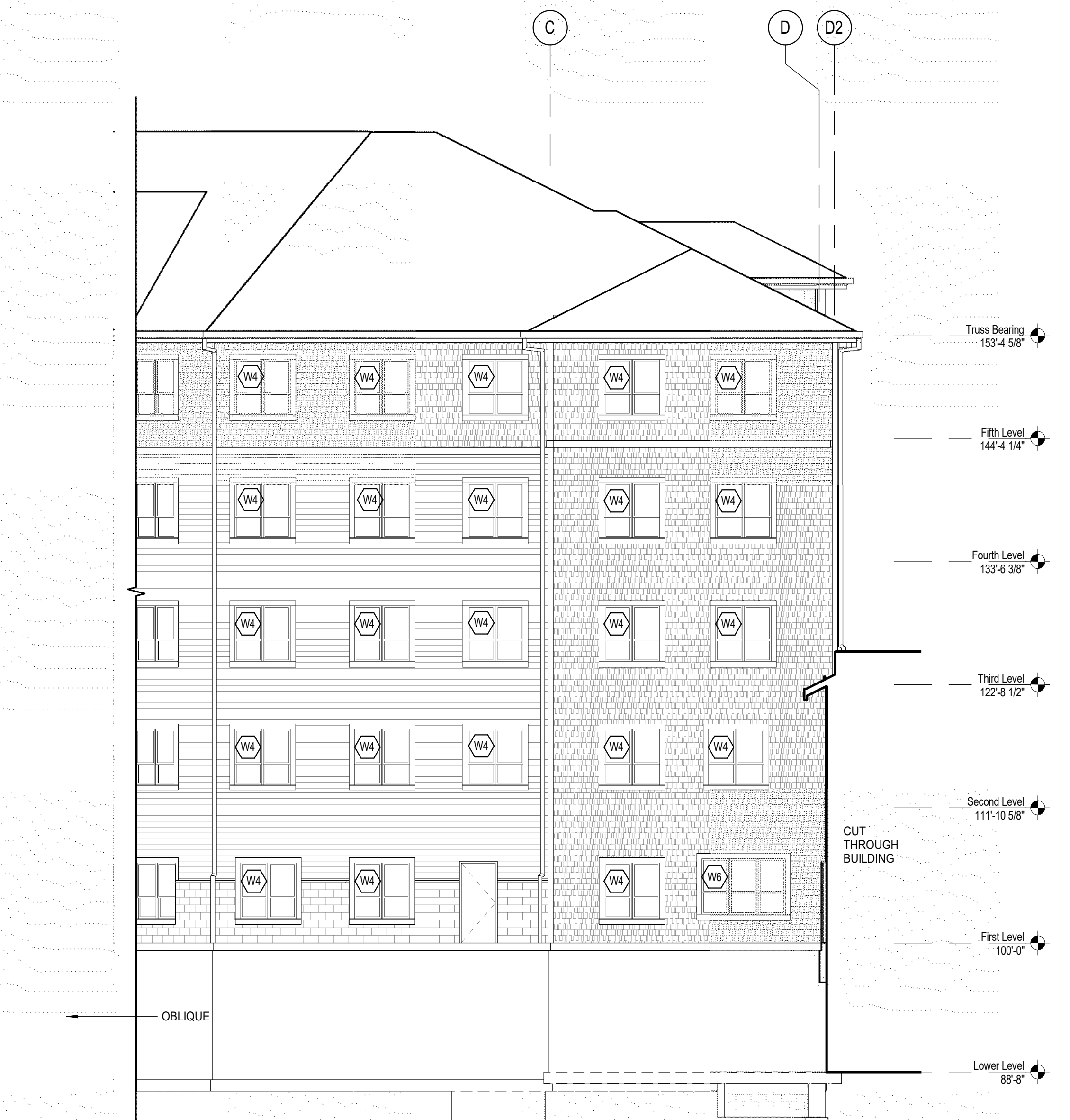
7 EXTERIOR ELEVATION- AREA D (S) A3.4 1/8" = 1'-0"
