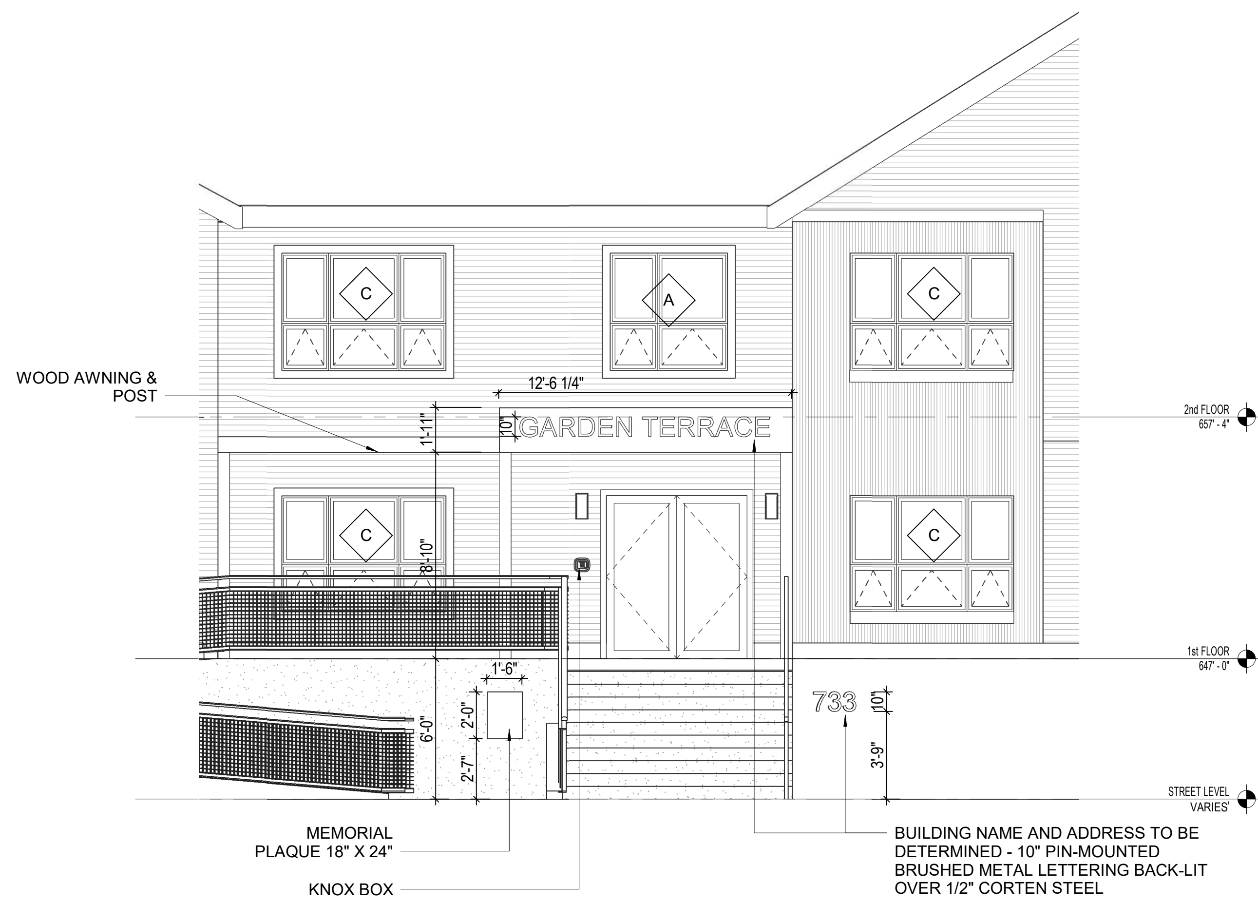
4 BUILDING SIGNAGE AT NORTH ELEVATION SCALE: 1/4" = 1'-0"
