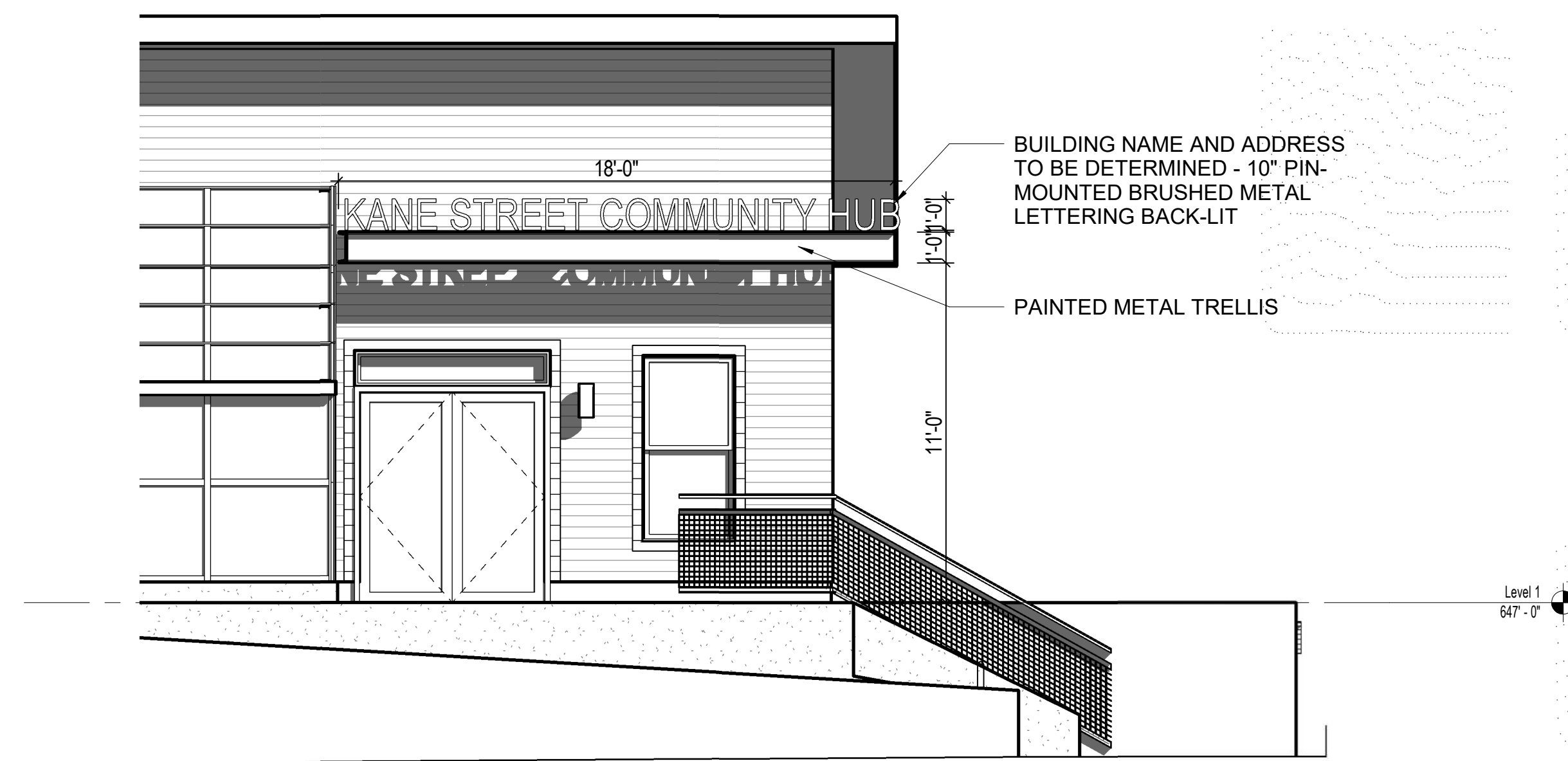
2 BUILDING SIGNAGE @ SOUTH ELEVATION SCALE: 1/4" = 1'-0"
