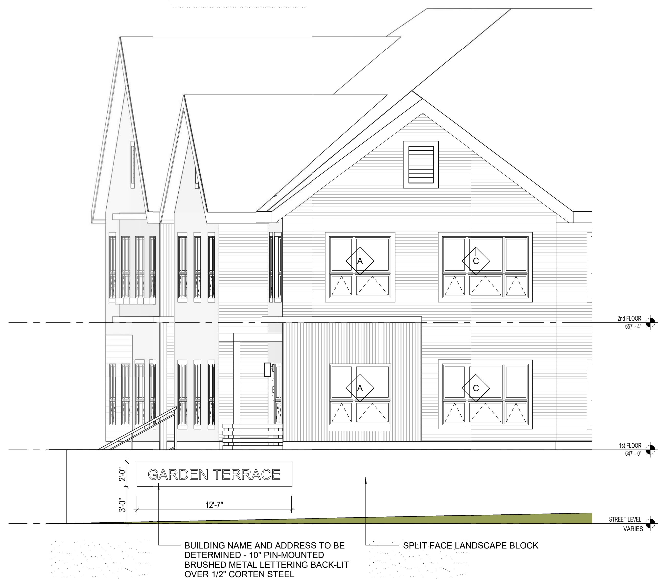
3 BUILDING SIGNAGE AT SOUTHEAST ELEVATION SCALE: 1/4" = 1'-0"
