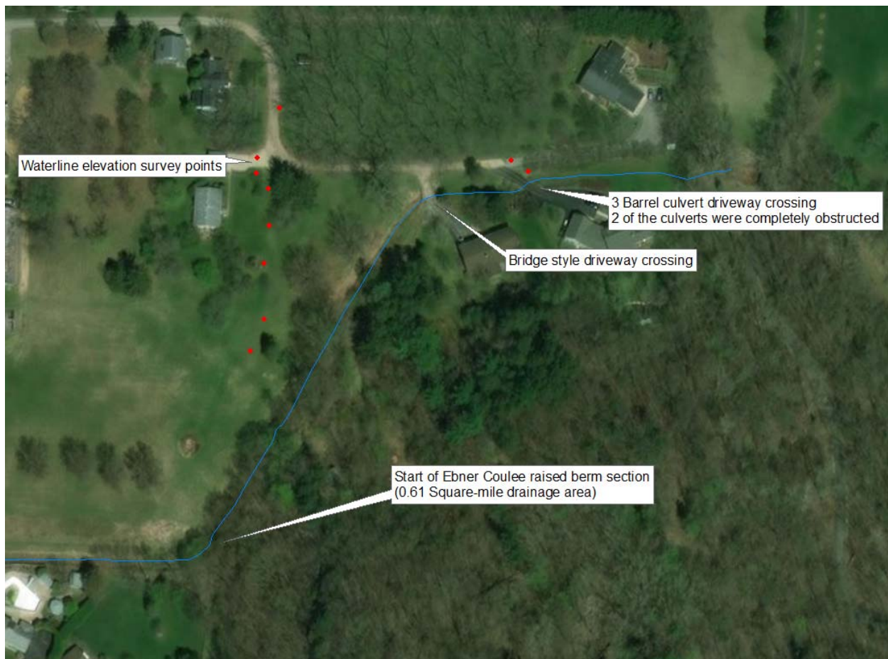
Figure 1. Upstream End of Channelized Portion of Ebner Coulee
