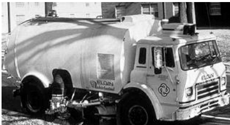
Street sweeping removes pollutants and sediments on the street to reduce pollutants entering receiving waters
