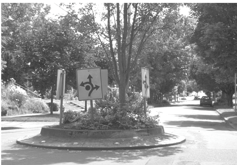
Traffic circle on local residential street [note: excessive signage can detract from appearance and may not always be necessary]
