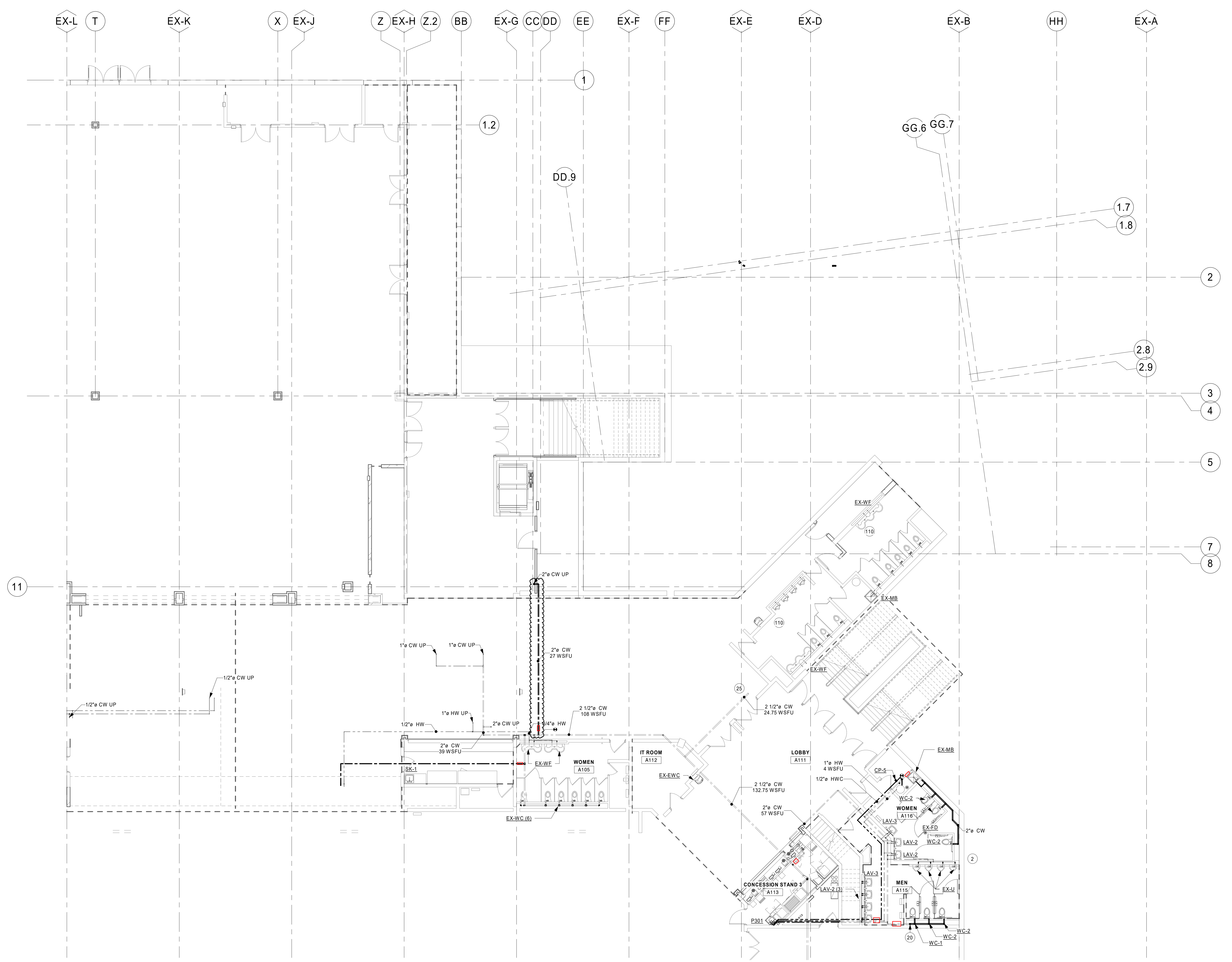
1 ARENA LEVEL DOMESTIC WATER - AREA B 1/8" = 1'-0"
