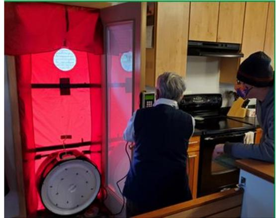
A blower door is used to measure how leaky the house is by depressurizing it and blowing air out of the house. This in turn pulls air in through all the gaps and cracks, helping to locate them.
