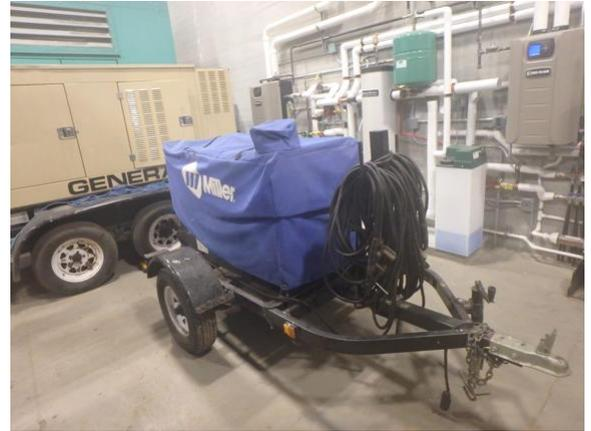
Used for welding and thawing frozen pipes.
