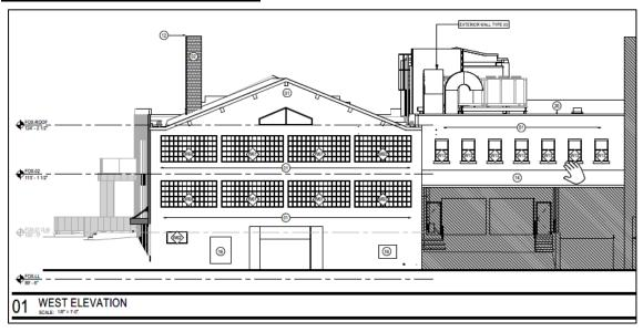
Original window openings will be restored with grid muntins or double-hung windows. There is also a trapezoidal window in the upper portion of this facade that was uncovered during demolition. This opening will be restored.
