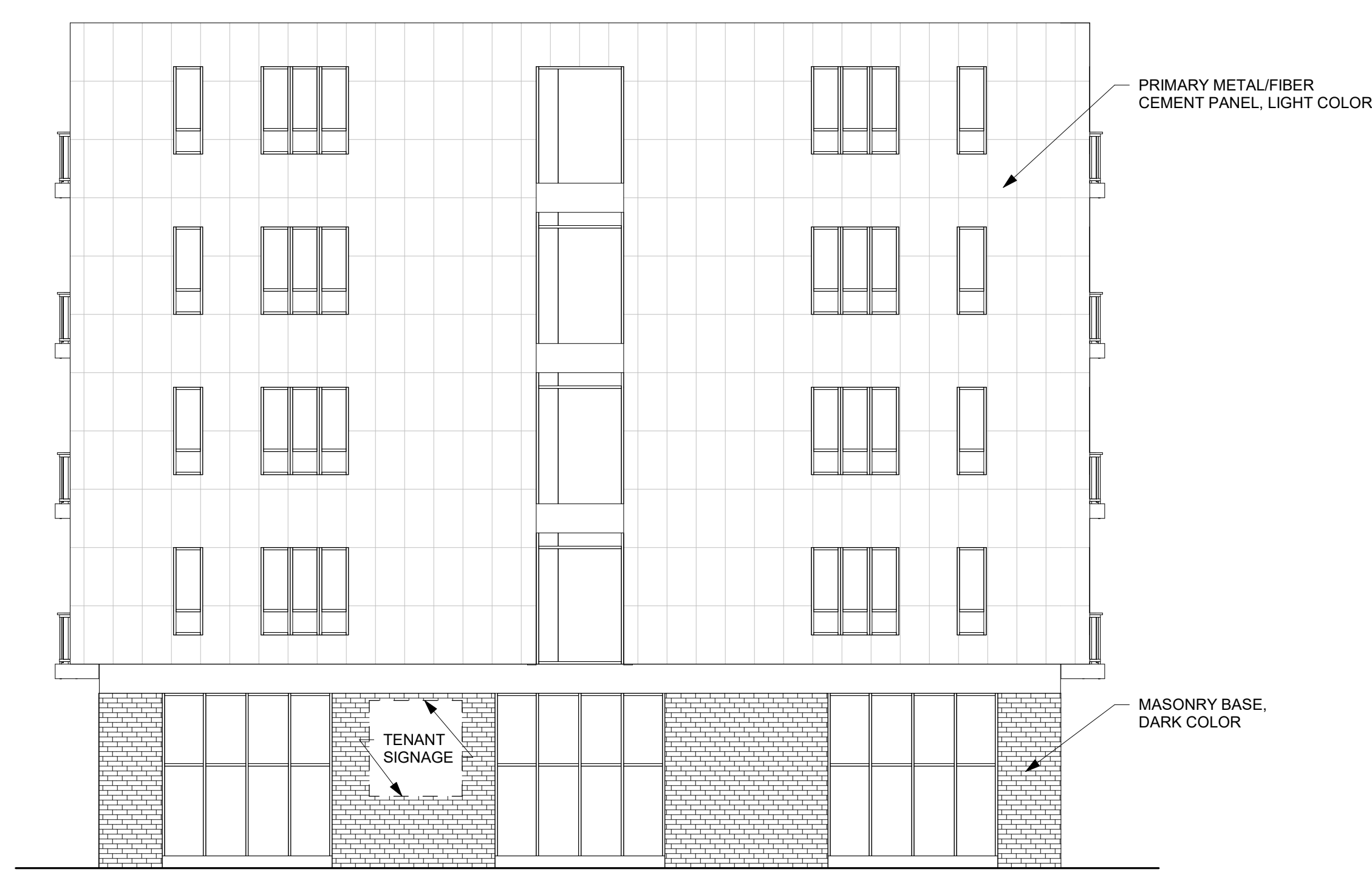
5 WEST BUILDING - NORTH ELEVATION 1/8" = 1'-0"
