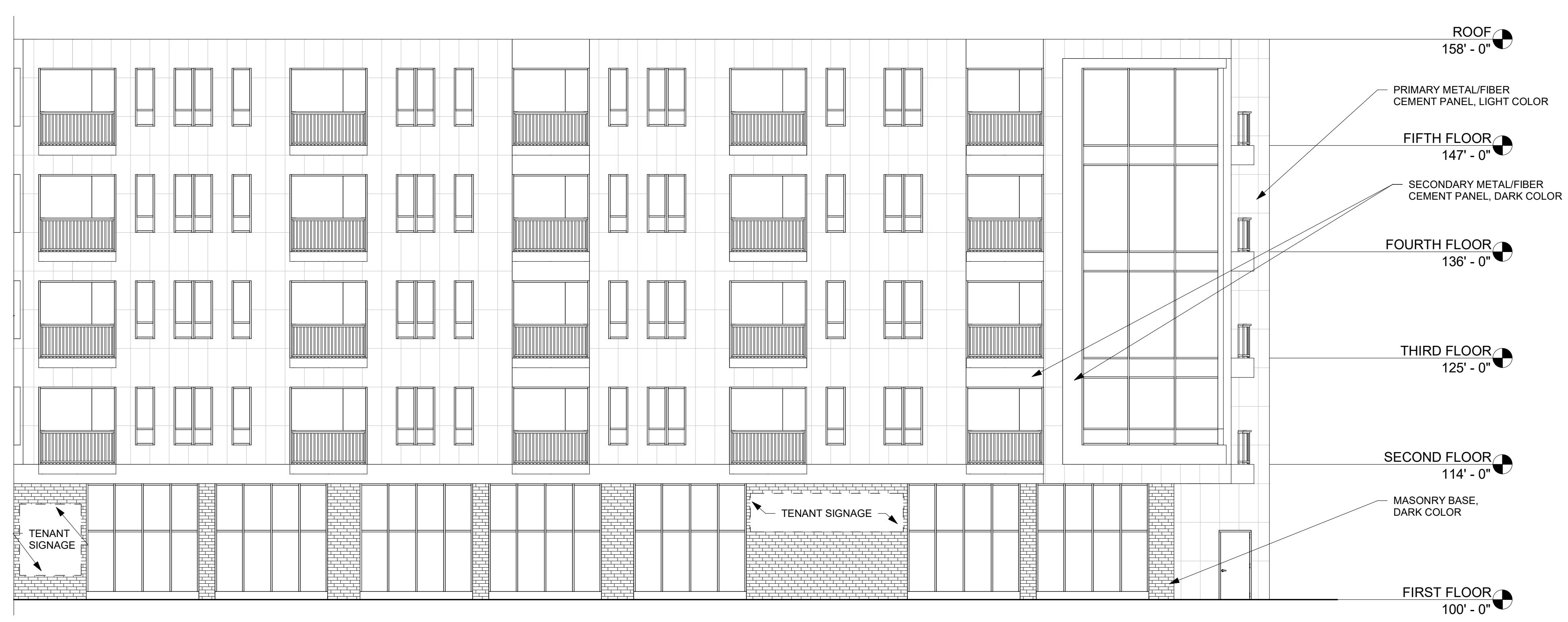
2 WEST BUILDING - WEST ELEVATION B 1/8" = 1'-0"
