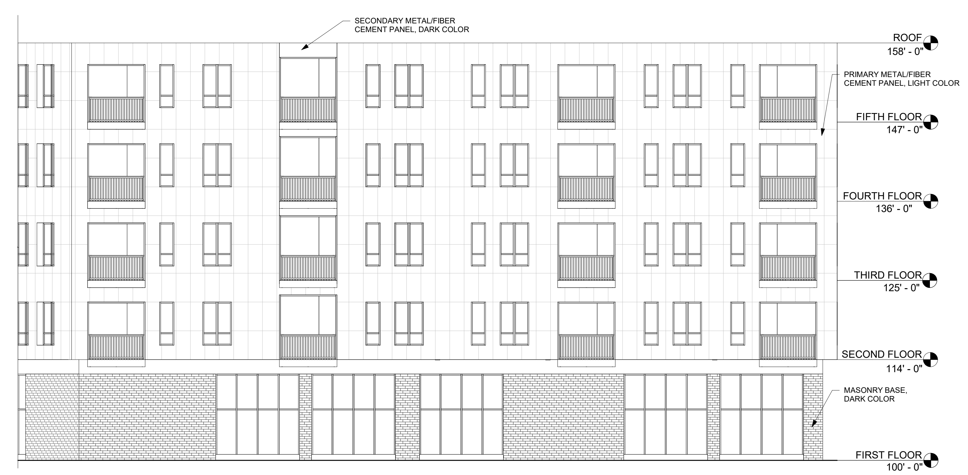
4 WEST BUILDING - EAST ELEVATION B 1/8" = 1'-0"
