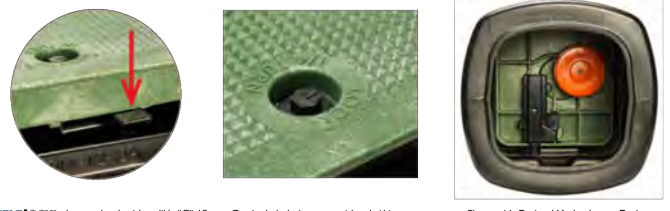
SELFLOCK closes and seals with audible "Click" Captive bolt device opens with only 1/4 turn Shown with Optional Marker Locate Device
