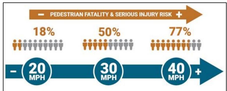
Figure 6: The risk of pedestrian serious injury or fatality in a crash with a motor vehicle increases dramatically between 20 and 40 miles per hour.
