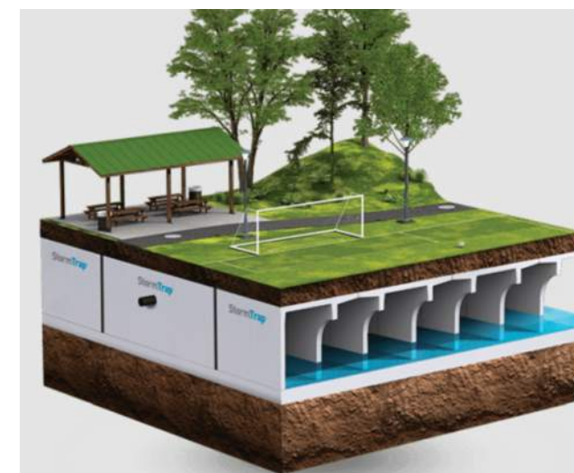
FIGURE 3.4.2: Rendered view of subsurface water detention vaults
