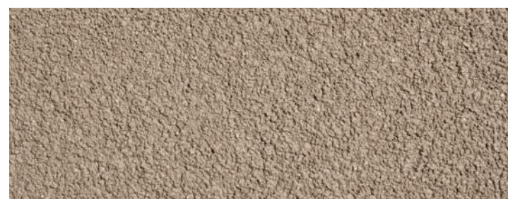
66 Exterior insulation and finishing system (EIFS)
