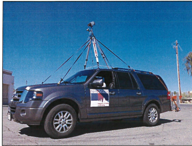
Figure 1 - Infrasense Infrared Survey Vehicle
