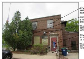
REMOVE GLASS BLOCK & INFILL MASONRY, PREP OPENING FOR NEW WINDOW (TYP.)
