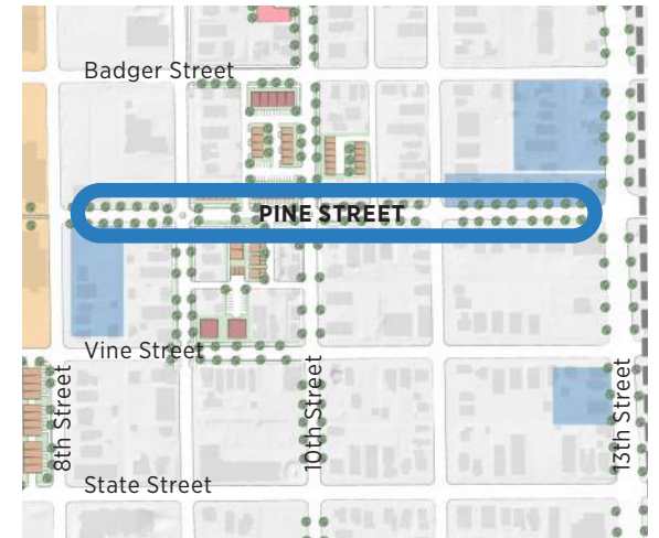
Pine Street, between 8th Street and 13th Street, can be adapted to a woonerf, meaning that traffic is designed for a pedestrian speed.
