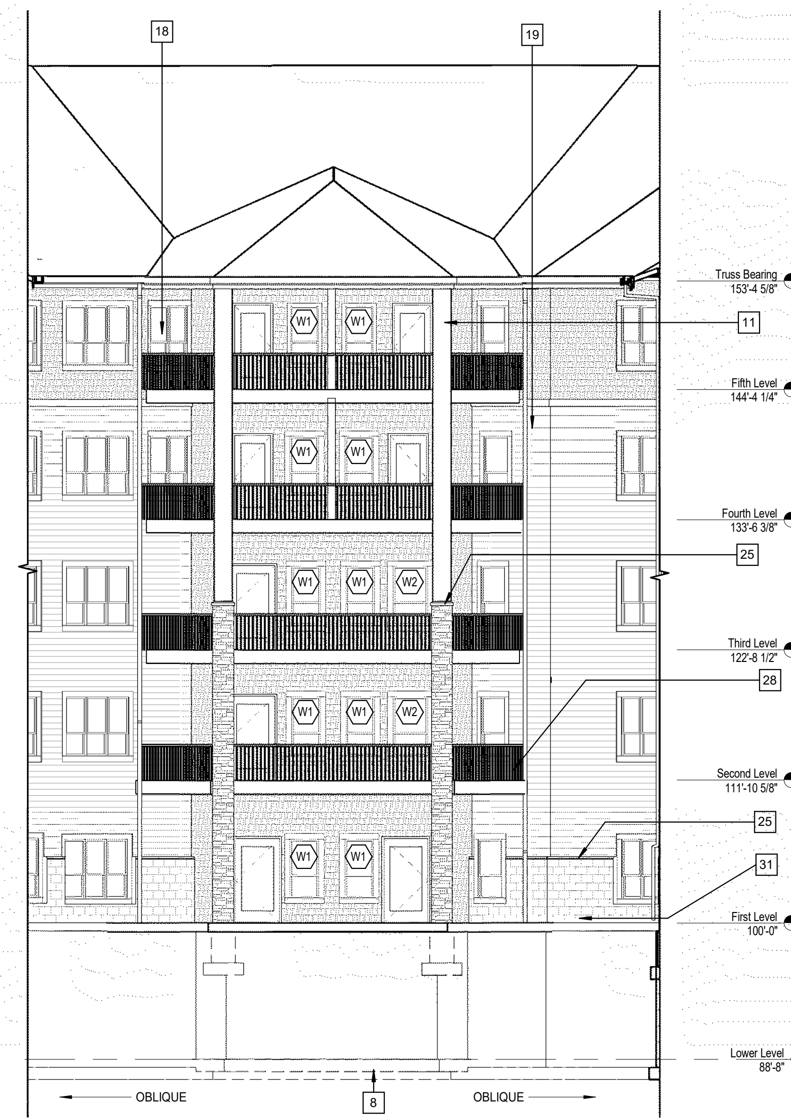
3 A3.3 EXTERIOR ELEVATION 1- AREA D (E) 1/8" = 1'-0"
