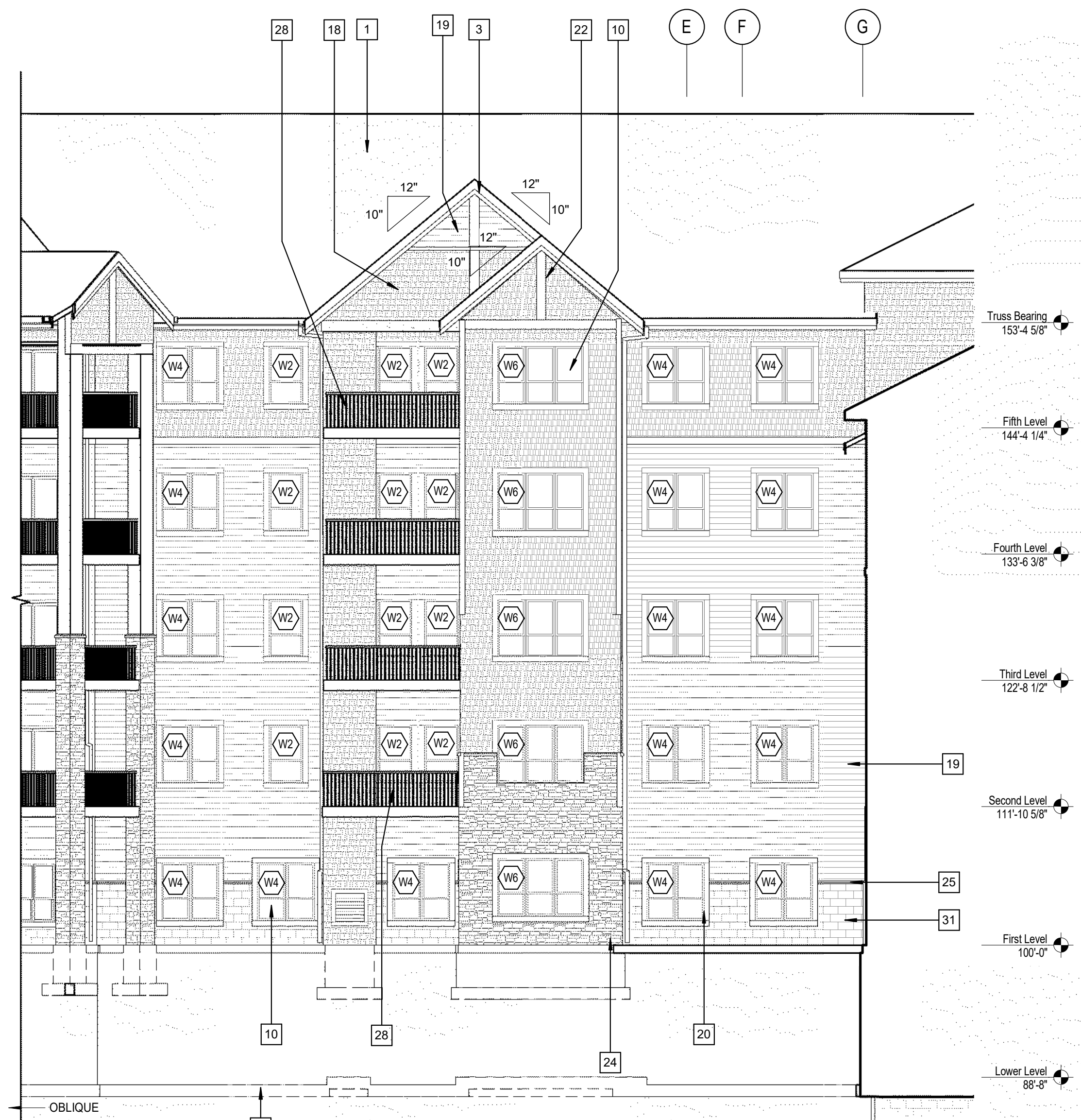
1 A3.3 EXTERIOR ELEVATION- AREA C (S) 1/8" = 1'-0"
