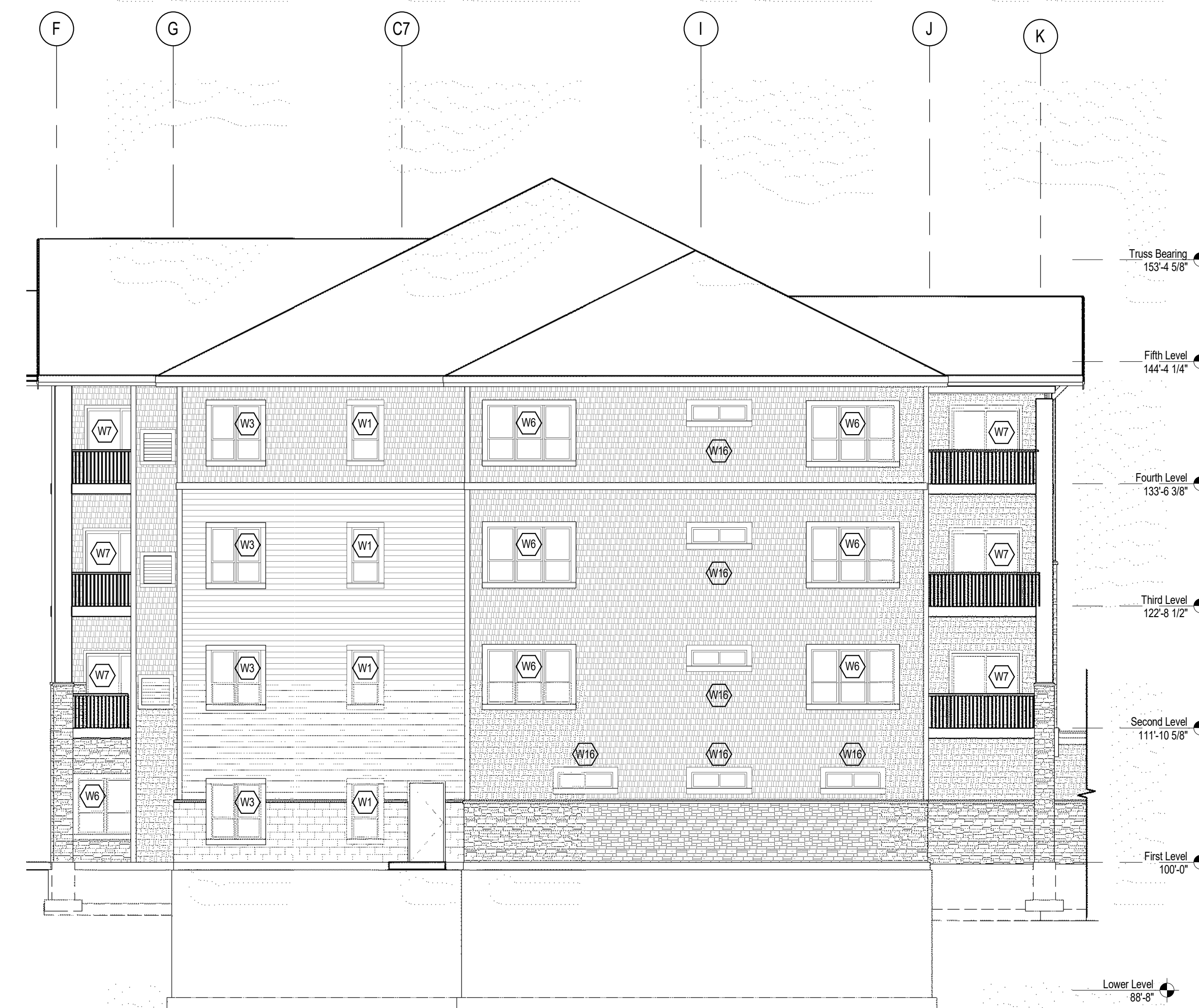
7 EXTERIOR ELEVATION- AREA A (S) 1/8" = 1'-0"
