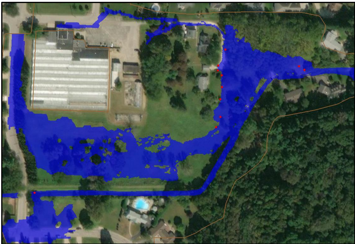
Figure 9 – SRH2D Inundation at Floral Lane – 300 cfs
