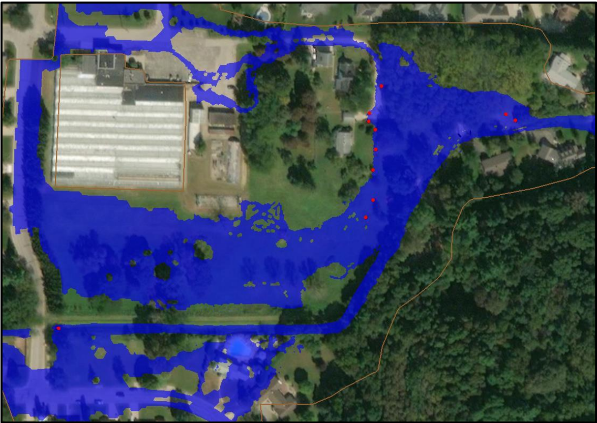
Figure 11 – SRH2D Inundation at Floral Lane – 500 cfs
