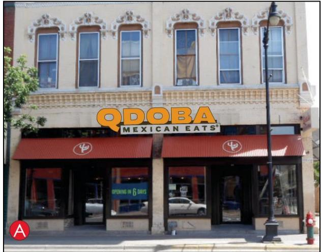
The Pearl Street wall sign will be 2'-0" in height and 9'-5" in width. It consists of black aluminum panels with a translucent acrylic face that is LED illuminated. It will be attached to the building with aluminum tieback clips and mounting fasteners via a large aluminum plate.
