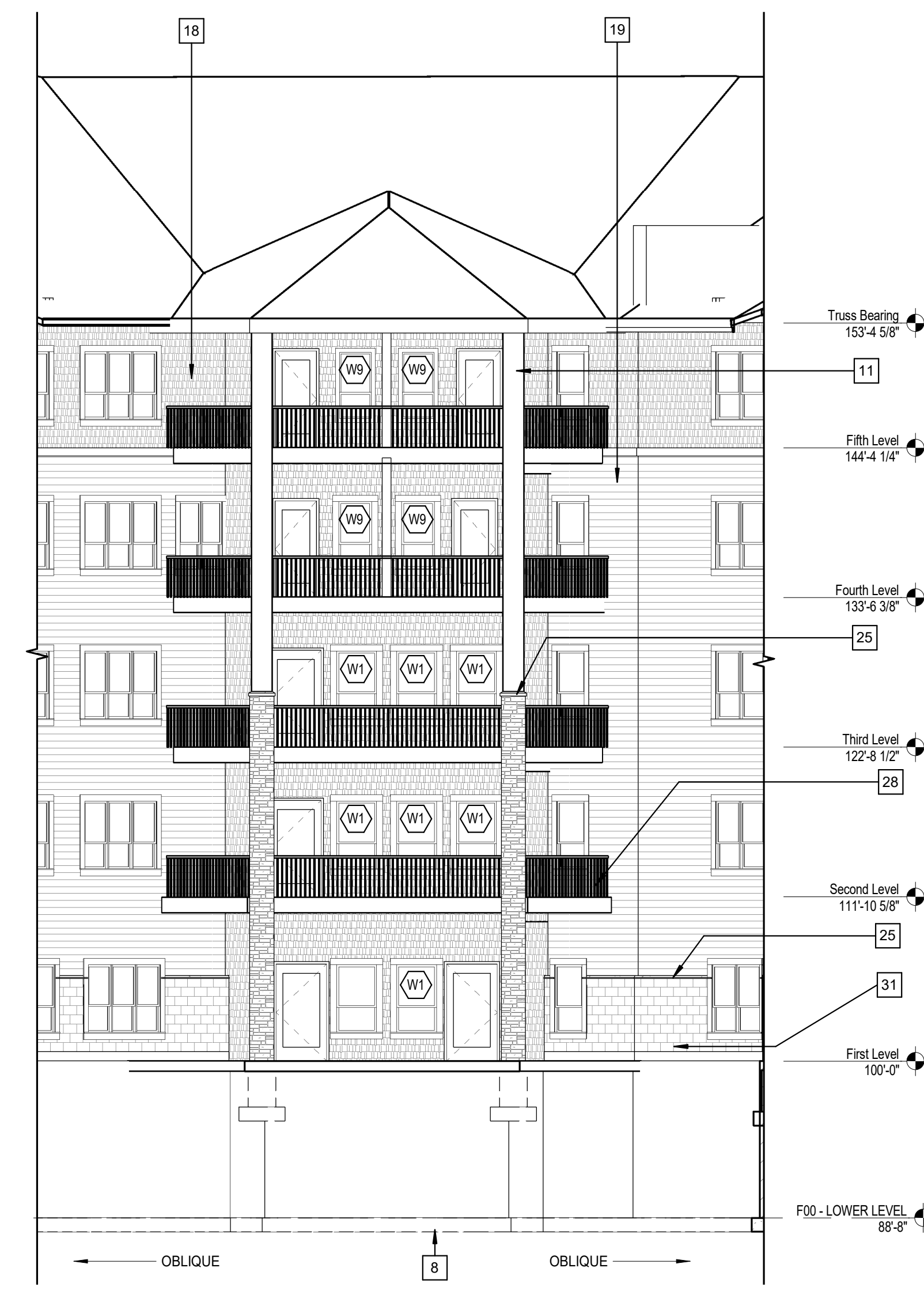
3 A3.3 EXTERIOR ELEVATION 1- AREA D (E) 1/8" = 1'-0"
