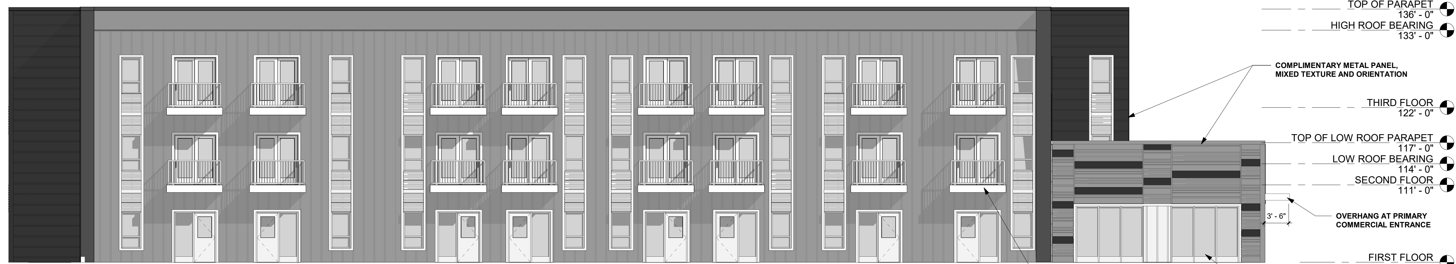
1 EAST ELEVATION 1/8" = 1'-0" TOTAL FACADE AREA - 5,538 SF TOTAL FENESTRATION REQUIRED - 5,538(0.2) = 1,107 SF TOTAL FENESTRATION PROVIDED = 1,800
