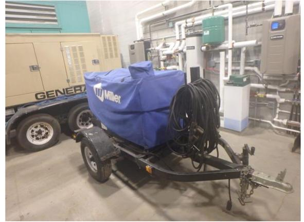
Used for welding and thawing frozen pipes.
