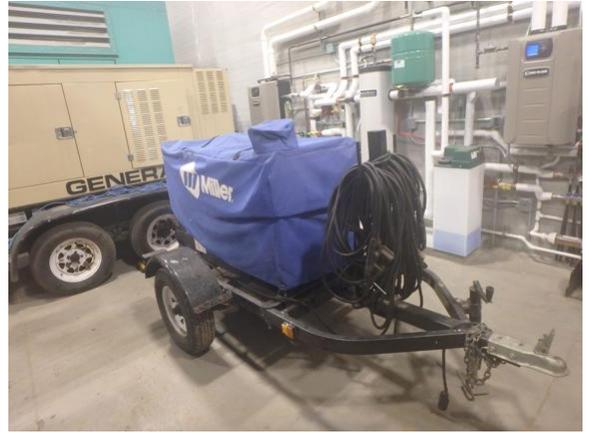
Used for welding and thawing frozen pipes.
