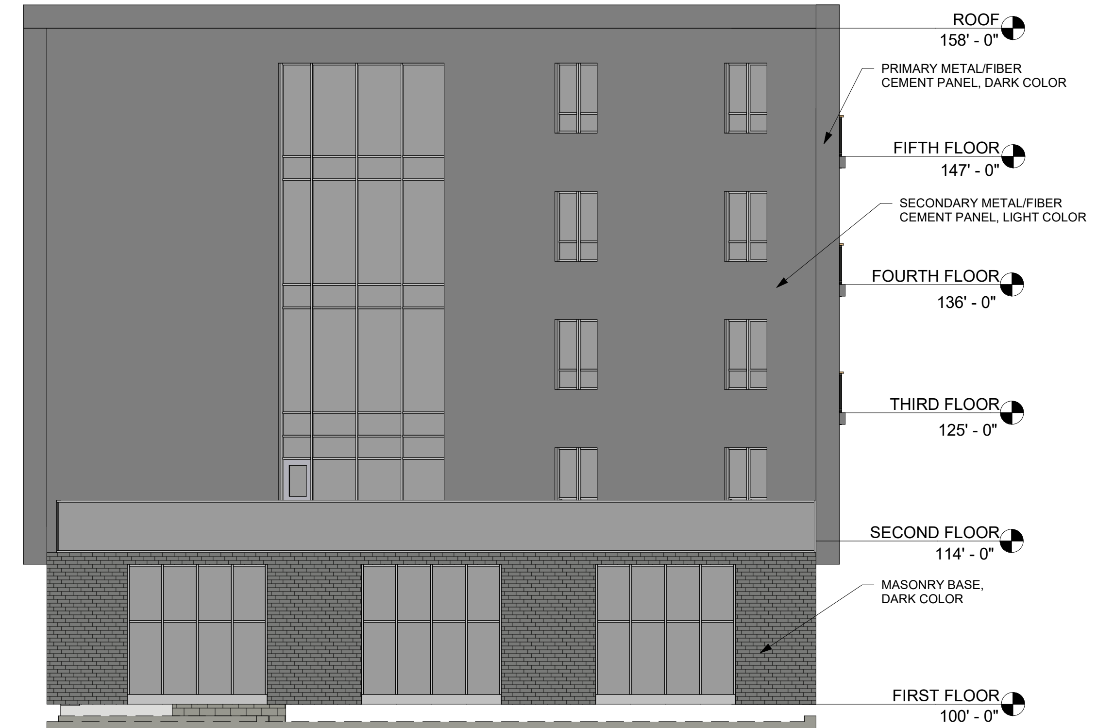
2 EAST BUILDING - NORTH ELEVATION 1/8" = 1'-0"
