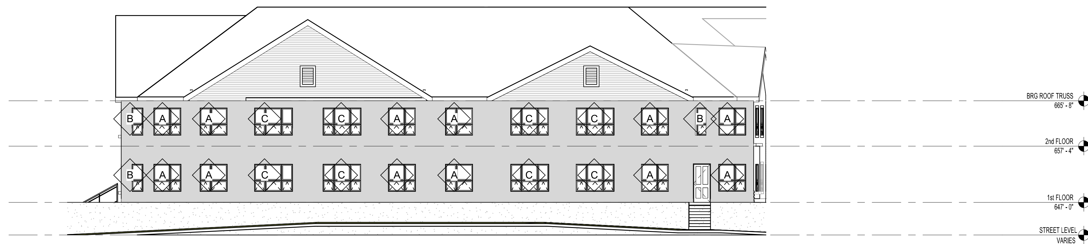
3 SOUTH ELEVATION - street facing facade 20% study SCALE: 3/32" = 1'-0"
