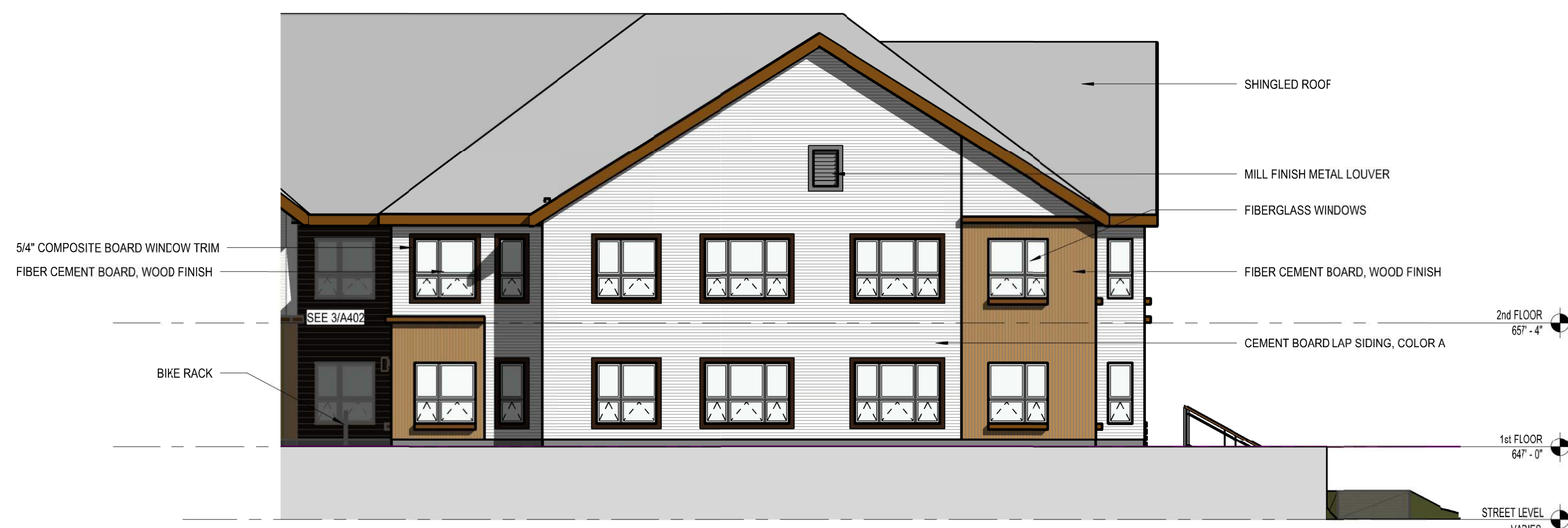
2 SOUTHWEST ELEVATION SCALE: 1/8" = 1'-0"
