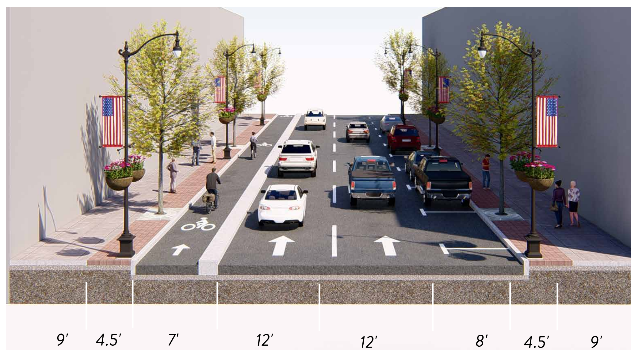
ALTERNATE: CURB SEPARATING BICYCLIST FROM STREET
