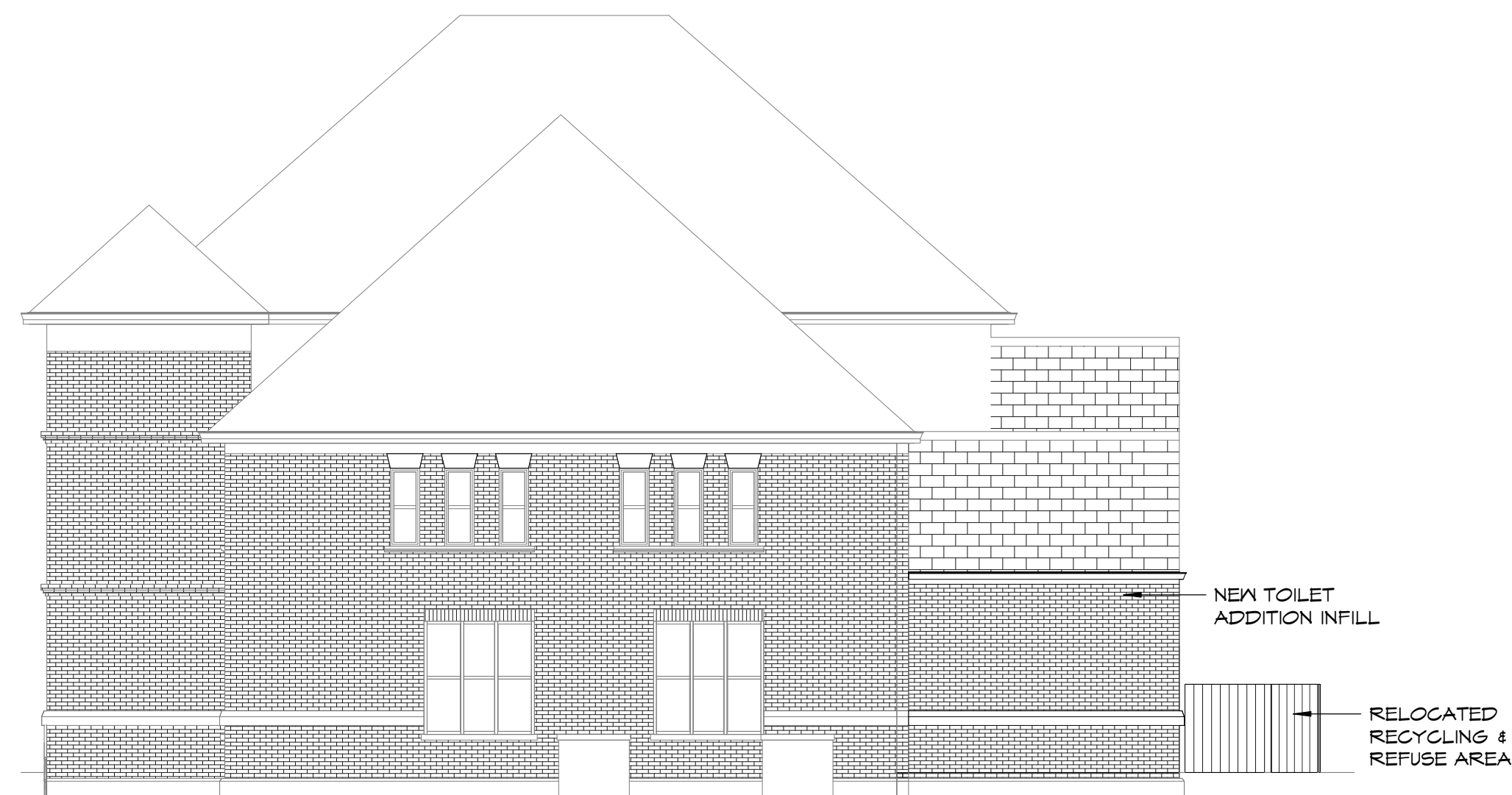
6 EAST ELEVATION - TOILET ADDITION 1/8" = 1'-0"
