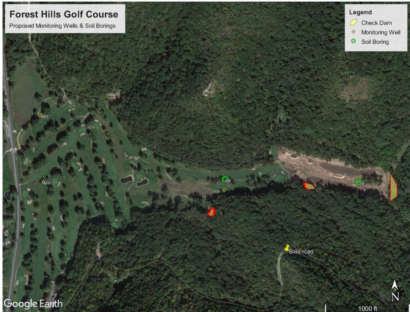
Figure 2 – Proposed Soil Borings and Monitoring Wells
