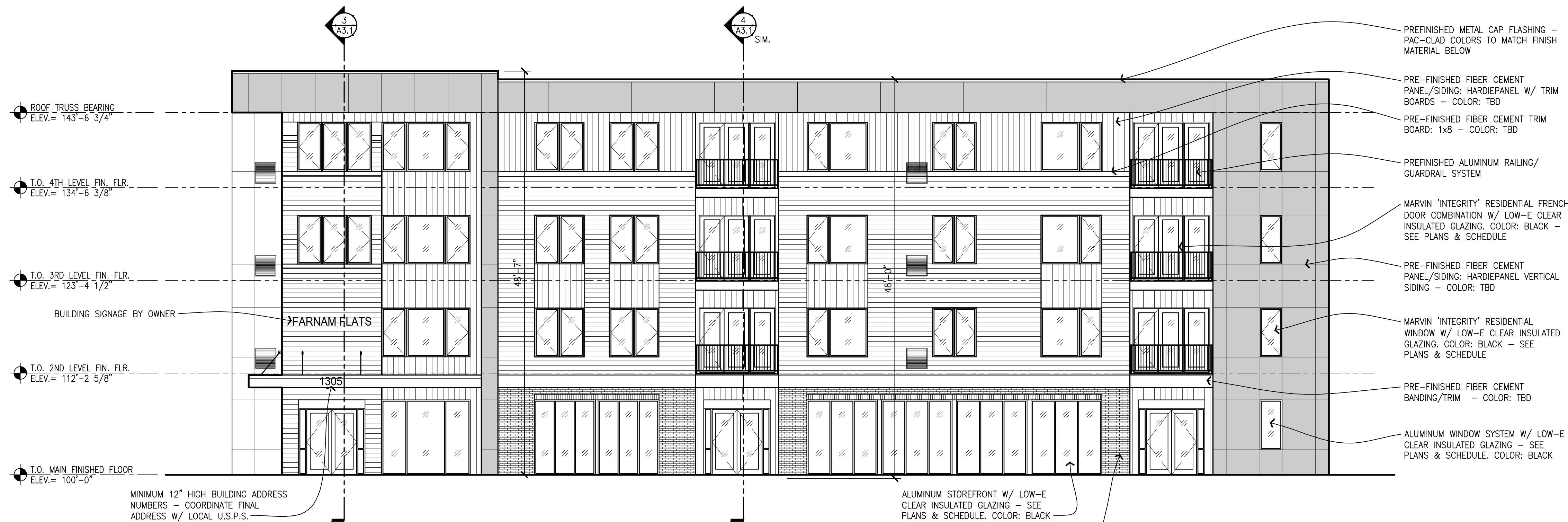
FARNAM STREET FACADE 1 SOUTH ELEVATION ORIGINAL SCALE: 1/8" = 1'-0"
