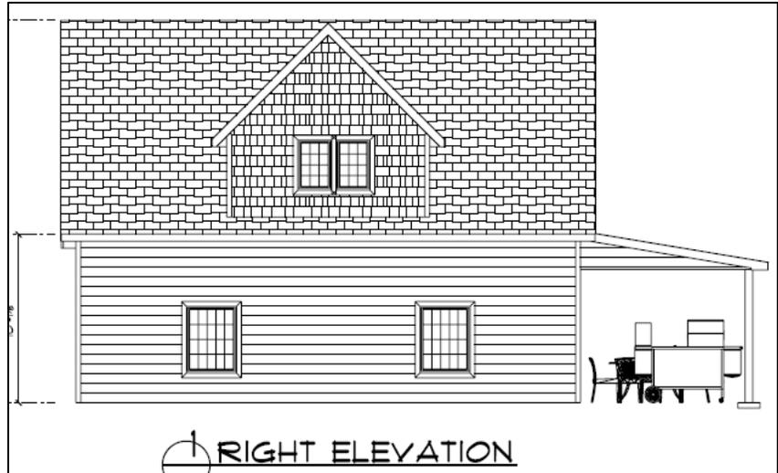
The roof will consist of asphalt shingles in order to match the house. The proposed use and location of LP Smart siding and shakes is intended to match appearance and look of the primary house.
