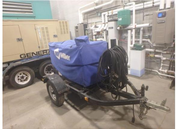
Used for welding and thawing frozen pipes.
