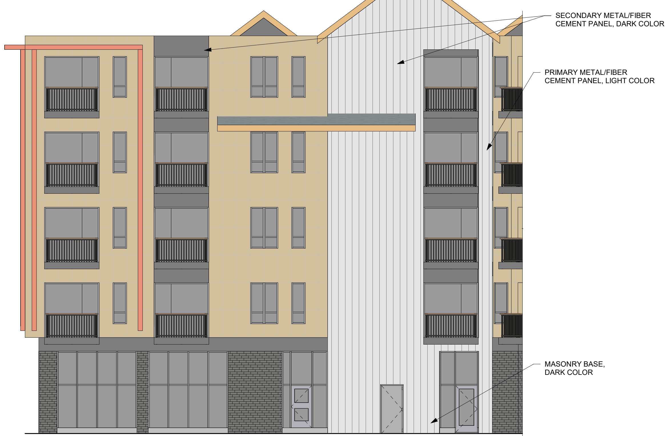
1 WEST BUILDING - WEST ELEVATION A 1/8" = 1'-0"
