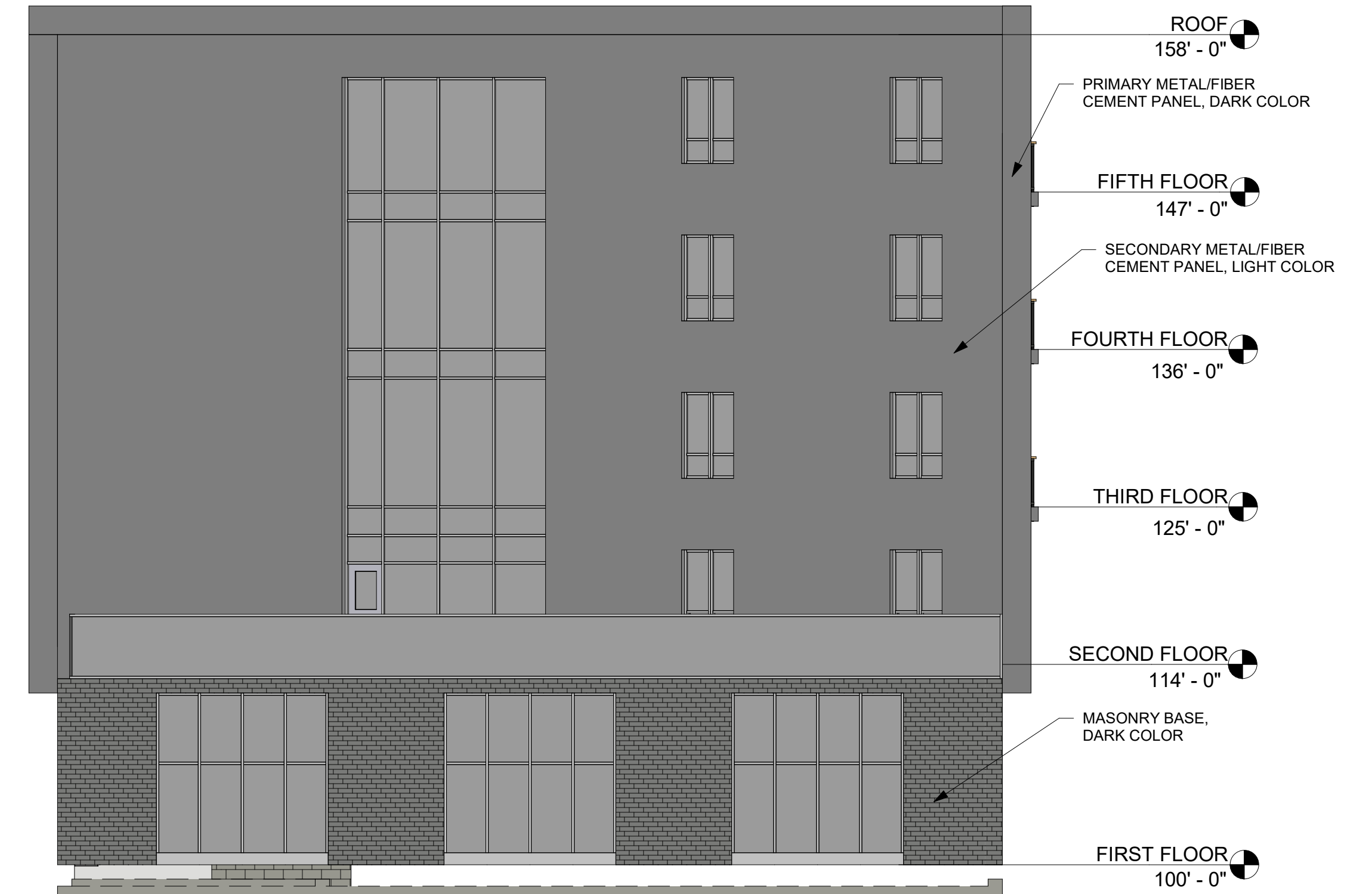
2 EAST BUILDING - NORTH ELEVATION 1/8" = 1'-0"
