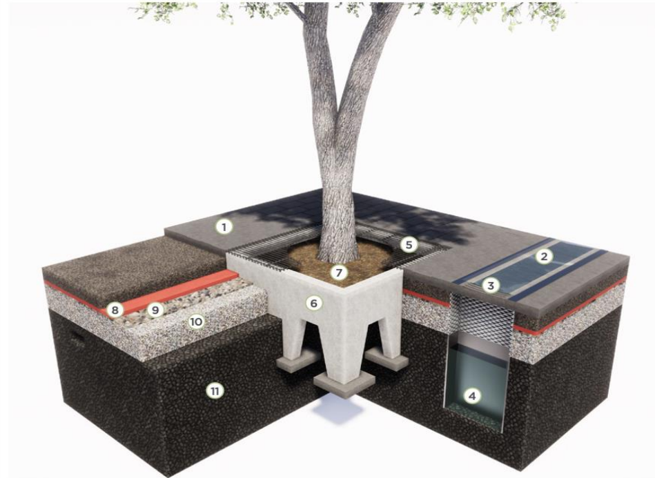
The Stockholm system (structural soil with biochar)
