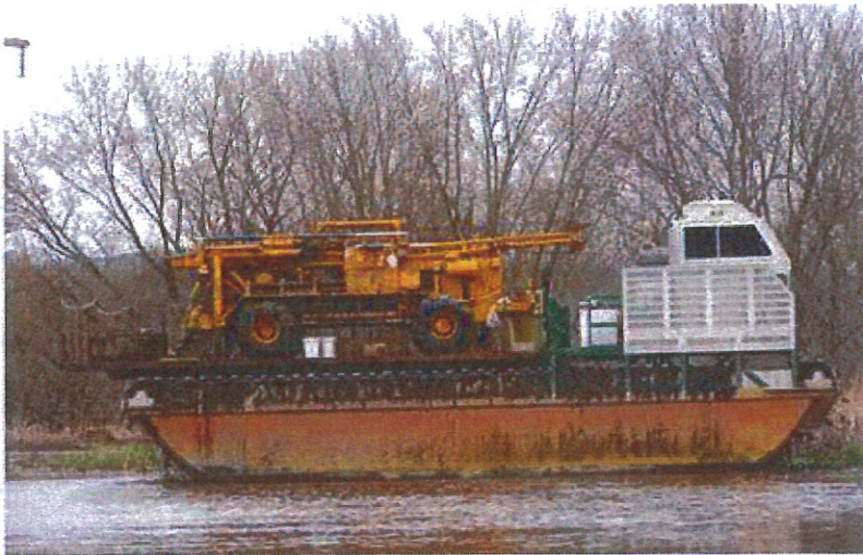
Marsh Buggy with soil boring rig
