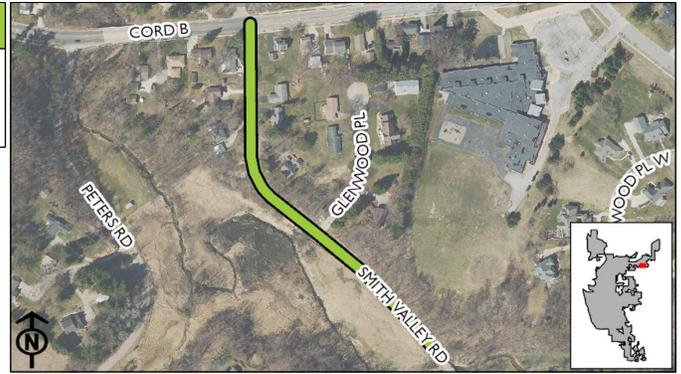
Installation of traffic calming measures, in the form of one to two speed tables, on Smith Valley Road. Placement and design to be done in-house by Engineering Department per City Traffic Calming Policy standards. Speed table(s) to be placed between CTH B and City Limits.
