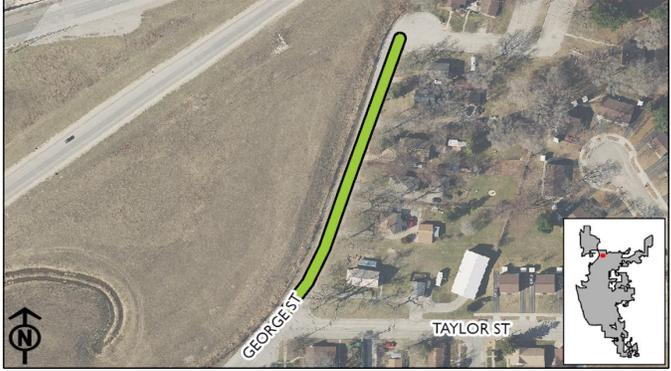
Complete NEW Curb & Gutter. Contract pave. Add new storm sewer. Add new sanitary (remove from Onalaska's), move water main.
