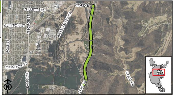
Install new 20-inch water transmission line to increase the water system capacity, pressure, and redundancy to La Crosse's north side.
