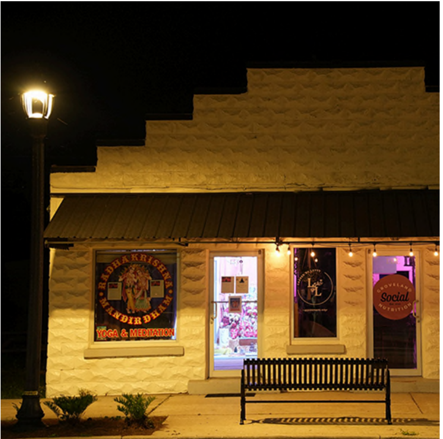
A downtown building has fully shielded, low-Kelvin streetlights to protect the night sky. Photos by Steven Miller Photography.
