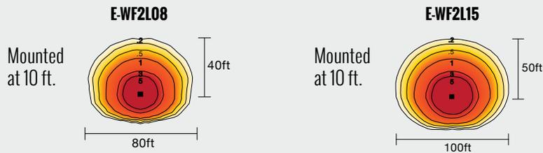
All published photometric testing performed to IESNA LM-79-08 standards by a NVLAP certified laboratory. Fixture photometry was completed on a single representative fixture.
