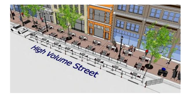
5. Diagram of Cafe zone that includes a "soft street closure" that allows fire, delivery and bicycle access in a 20' lane down the middle.
