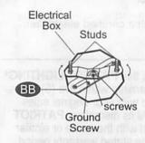
3. Firmly attach the fixture ground wire (bare copper) to the mounting bracket (BB) with the ground screw (by wrapping around the ground screw) and then connect it to the house supply ground wire with a wire nut. Connect black wire from fixture (A) to black wire in electrical box and connect the white wire from fixture (A) to white wire in electrical box. Use supplied wire nuts (AA) for all wire connections.
