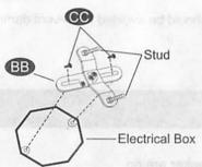
2. Position mounting bracket (BB) so that the fixture will be hung properly once it is mounted to the wall. Tighten the screws to hold in place.
