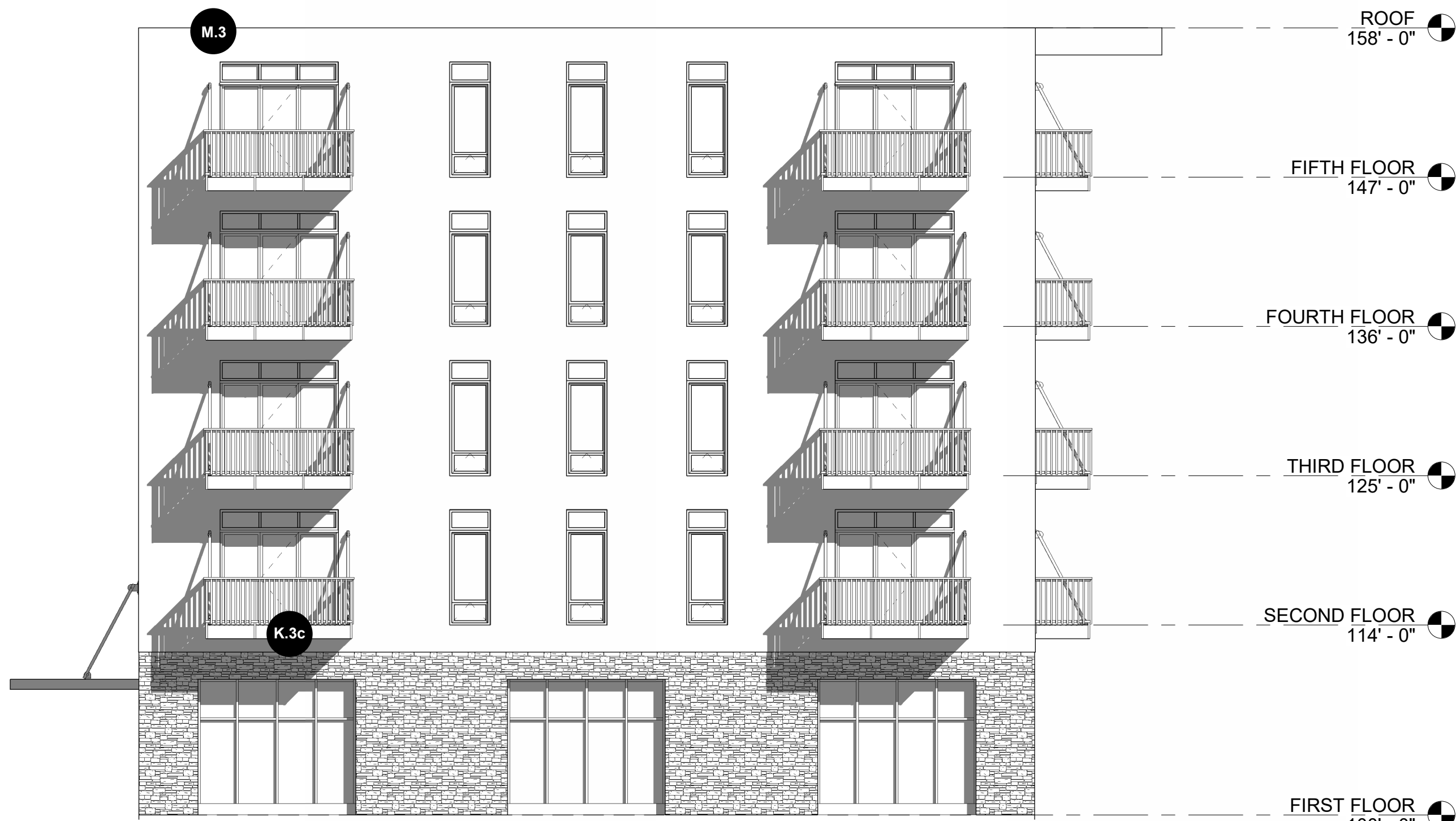
3 WEST BUILDING - NORTH ELEVATION1 1/8" = 1'-0"
