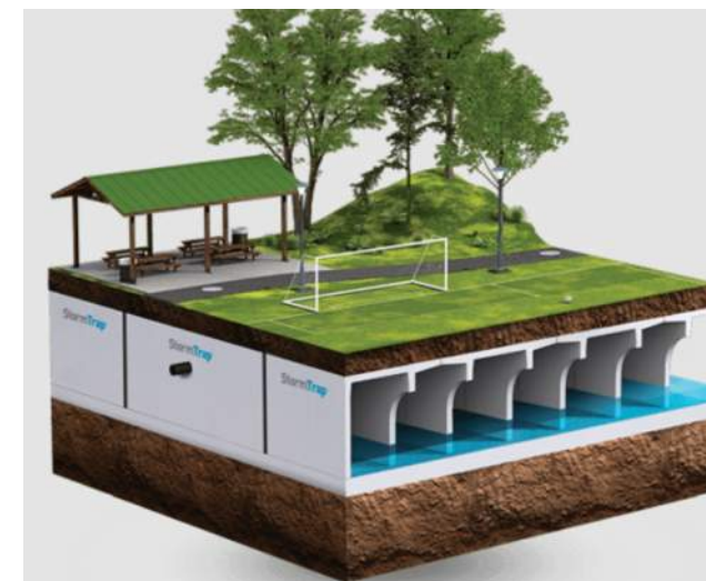
FIGURE 3.4.2: Rendered view of subsurface water detention vaults
