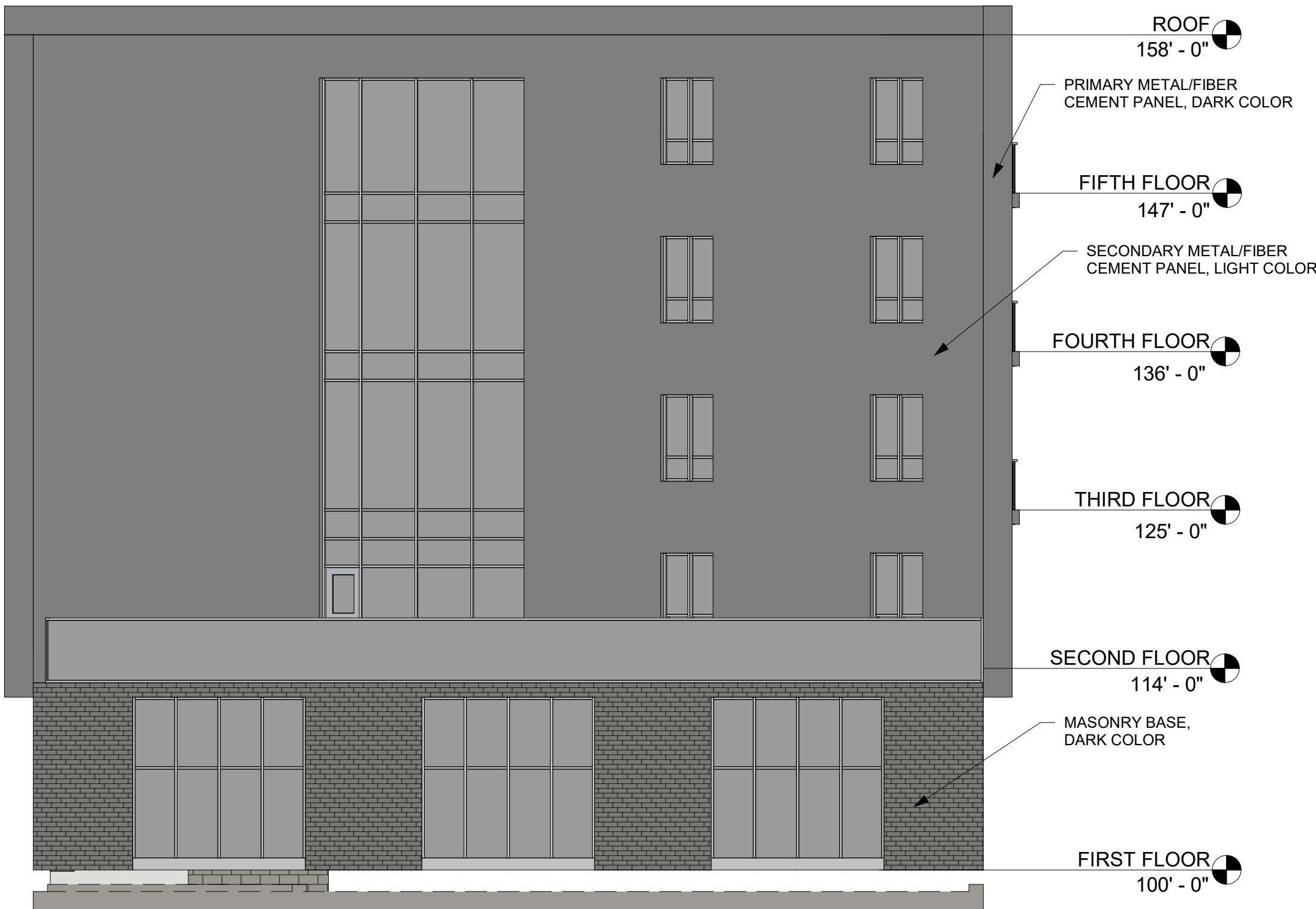
2 EAST BUILDING - NORTH ELEVATION 1/8" = 1'-0"
