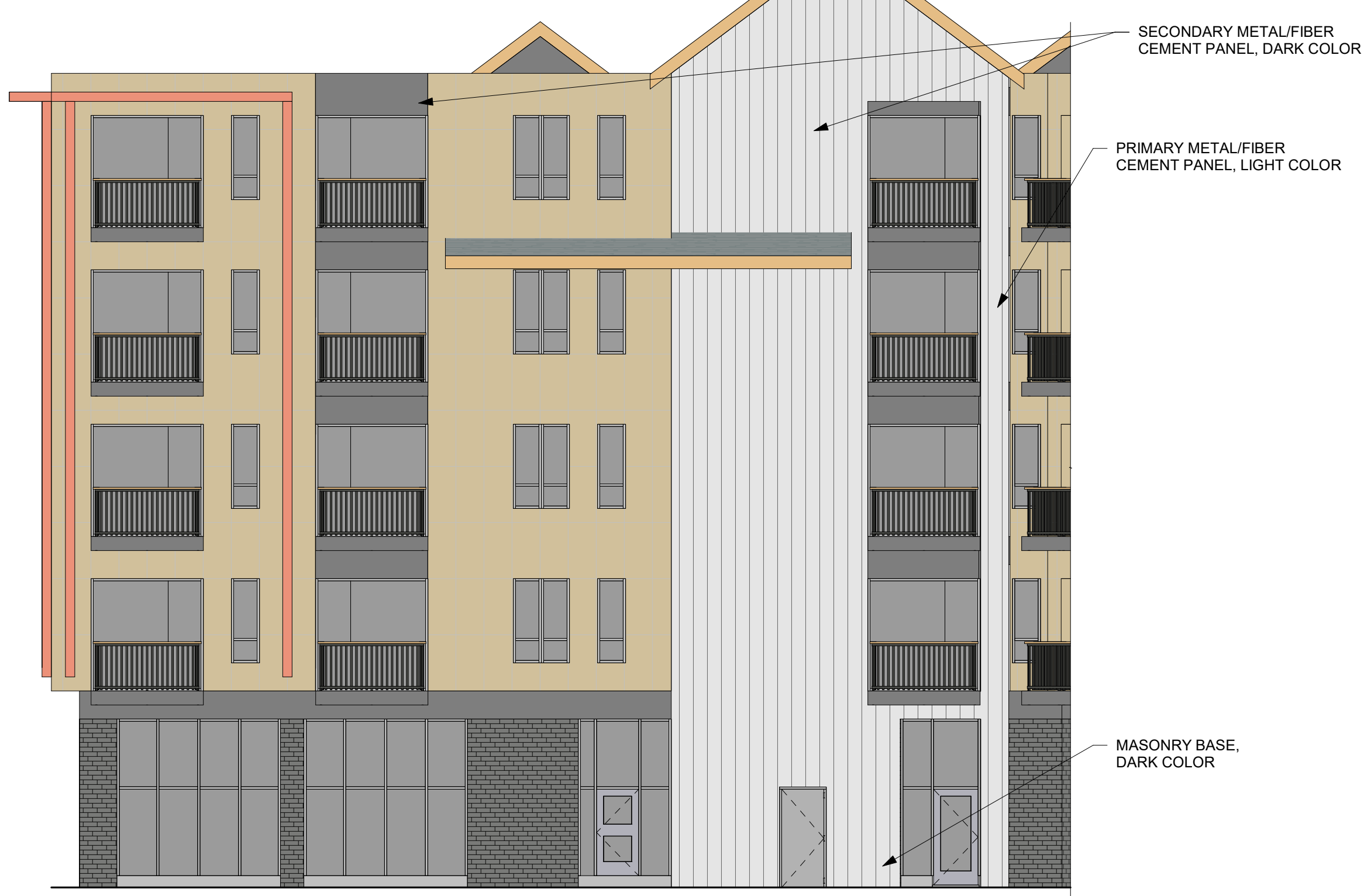
1 WEST BUILDING - WEST ELEVATION A 1/8" = 1'-0"
