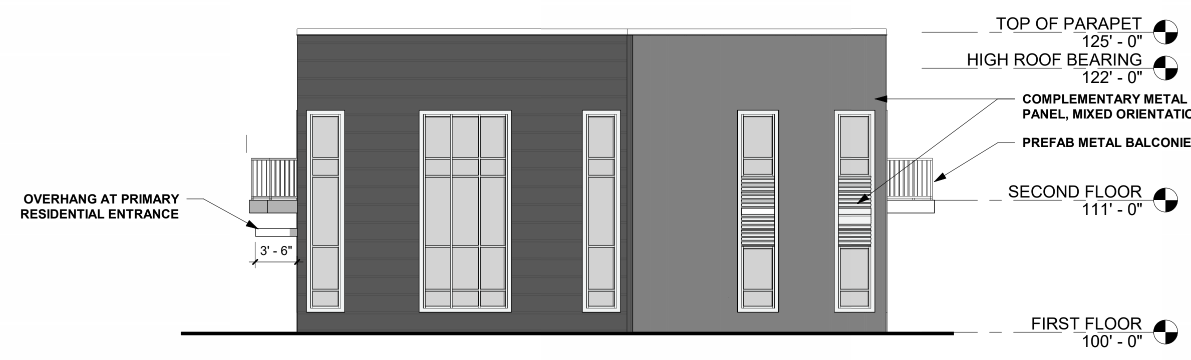
3 SOUTH ELEVATION 1/8" = 1'-0" TOTAL ELEVATION AREA = 1,240 SF TOTAL FENESTRATION REQUIRED = 1,240(0.2) = 248 SF TOTAL FENESTRATION PROVIDED = 251 SF
