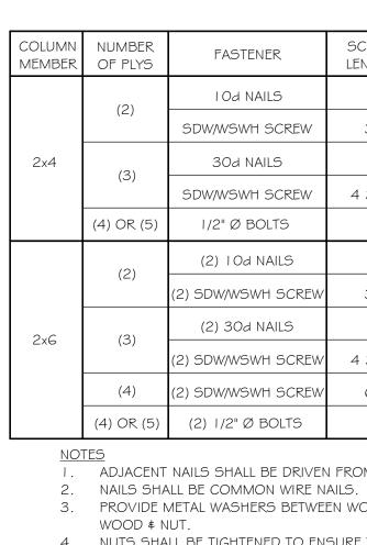
4. NUTS SHALL BE TIGHTENED TO ENSURE THAT FACES OF ADJACENT LAMINATIONS ARE IN CONTACT. 5. JACK/KING STUD PACKS SHALL ACT AS ONE COMBINED BUILT-UP COLUMN,
