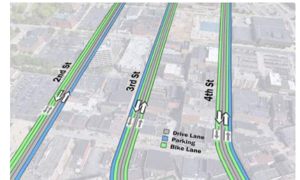
Scenario D: One-way pairs on 3rd and 4th become to two-way traffic to encourage commerce, long truck and bus movements, and bicycling-pedestrian safety and mobility
